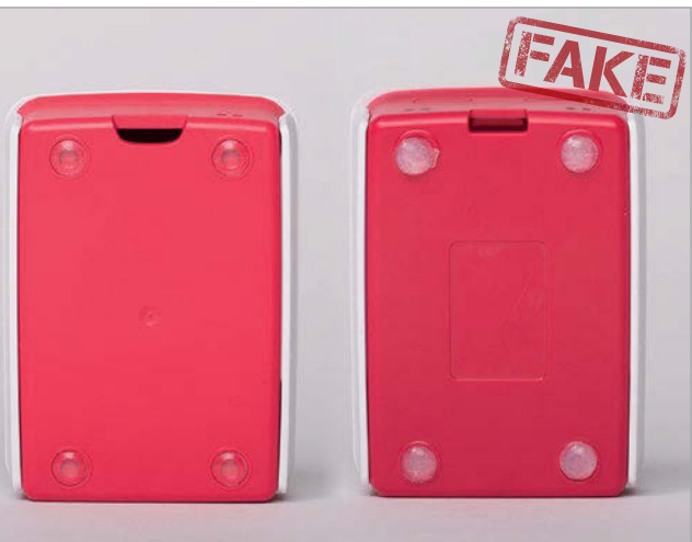
Above This fake case has two sets of light pipes Below The shoddy feet on this case are a clear sign of a fake
