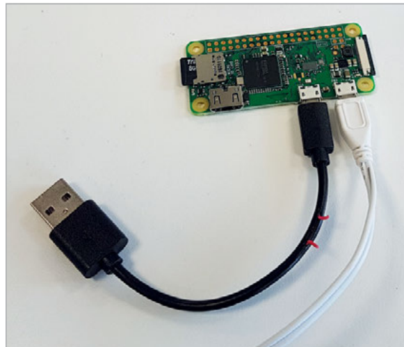
Left Use a modified cable to keep the Pi Zero W powered, even when the TV is switched off
