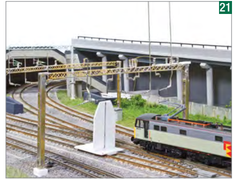
Gauges are one way of fitting register arm assemblies at a constant height from the rail right across a layout and avoiding inconsistencies that might damage pantographs.
