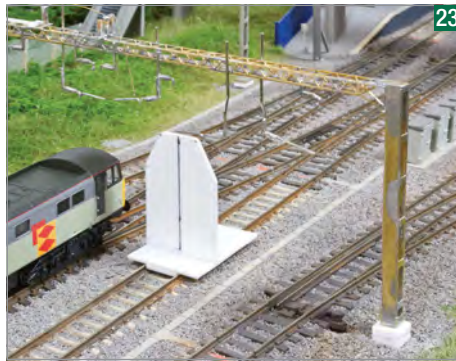
A centre-line was drawn on the register arm height gauge to position each arm. The top of the gauge is the width of a Dapol pantograph head.
