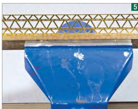
The bending former is placed against the lower edge of the half etched line and etched holes. Solder fills as much of the folding holes as possible.
