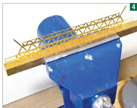
A small bench vice was used to hold etchings and bending formers securely when forming each bend. Use pieces of wood to protect the etch if it has serrated jaws.
