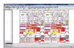
The production etch drawing (still in false colour). Two loos per sheet and space left over used for some other useful bits and pieces.
