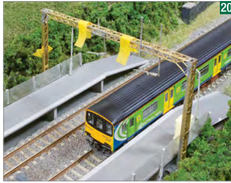
Masking tape has been used to mark in the track centre lines in the station area before the register arm assemblies were fitted.
