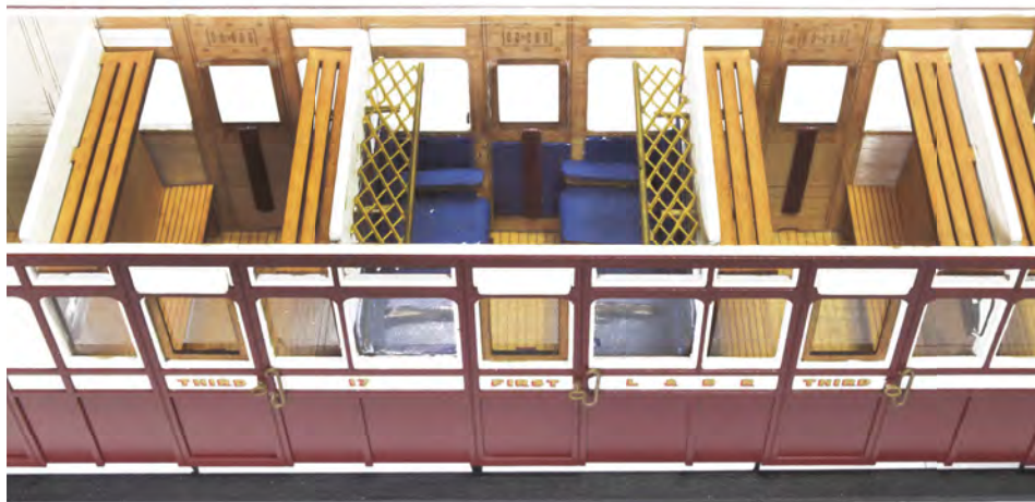
Upholstered first class non-smoking compartment and third class interior finish
