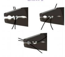
Position crimp and wire in pliers cup shaped hole. This is usually closest to handle. Squash crimp. Move squashed crimp to circle shaped hole at front of pliers, with cup facing sideways like a back to front "C" gently compress to form a ball. Test to ensure crimp is secure.
