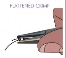
Position crimp gently with chainnose pliers, making sure that wires are tensioned correctly gently flatten crimp using pliers, so it remains in alignment with wire in a neat square shape. Test to ensure crimp is secure before proceeding.
