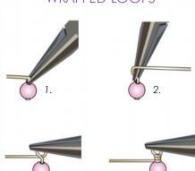
Using roundnose pliers grip wire above bead press with fingers to right angle. Place pliers in upright position and pull wire over top of pliers and back to right to form neat round loop. The size of your loop will vary on where you place the pliers on the wire.
