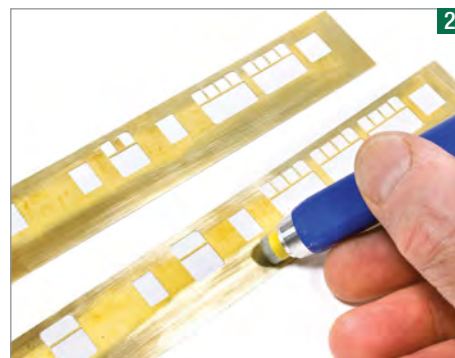
To give the adhesive the best chance of bonding styrene to brass, the inside of the sides are burnished and cleaned with a scratch pencil.
