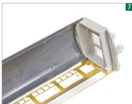
A closer view of the cab to roof to side assembly. A little filler was needed to finish the cab to roof join. The mix of materials makes choosing the right adhesives crucial.
