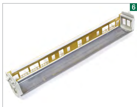
Assembly of the body progresses with both cab castings fitted together with one side. Note how the extra styrene strips help to locate and fix the brass sides.
