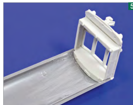
Care is taken to align the rain gutter of the roof moulding with that of the cab castings. Hold the two parts together as the CA glue dries.
