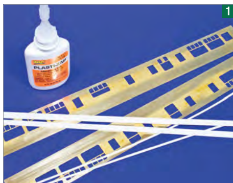
Strips of 20 thou' styrene are cut to fit the inside of the brass sides to add strength and act as a fixing point for the plastic roof.
