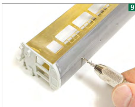
The vent holes are opened out with a larger diameter drill just slightly wider than the vent casting spigots. This allows for slight variation in the size of the spigots.
