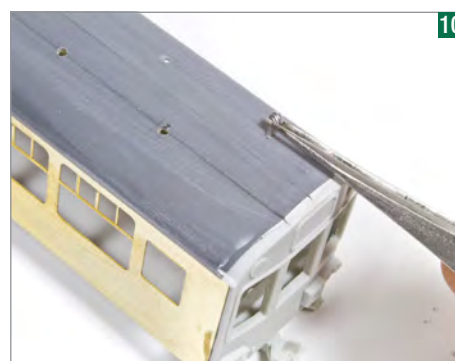
Shell vents are fitted with a spot of CA glue. The slightly larger hole also allows for some adjustment of position so they can be fitted in a perfect line.
