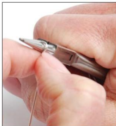
Forming a simple loop
