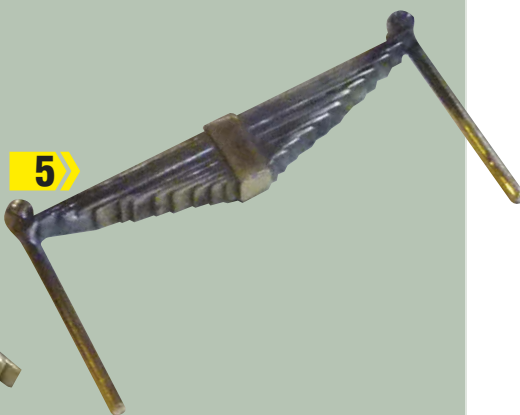
Spring hangers are made from brass rod with brass tube forming the retainers to finish.
