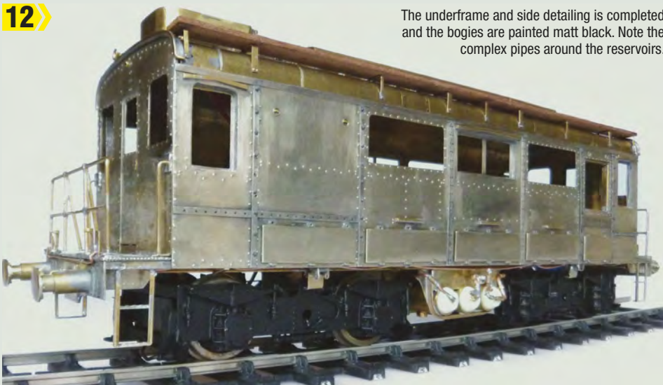
My simplified model of the Allen engine is built from plastic sheet, detailed with small brass pins and riveted sheet. It can be seen through the side windows and was enjoyable to make. Given time I'll add some more machinery.
