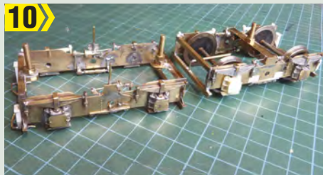
Axleboxes, spring detail, pipes and brake hanger detail is fitted, referring to photographs along the way.
