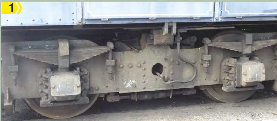
The bogie sides on the locomotive are hefty pieces of steel. Roller-bearing axleboxes weren't widely used at the time, as seen here with these oil-filled axleboxes.
