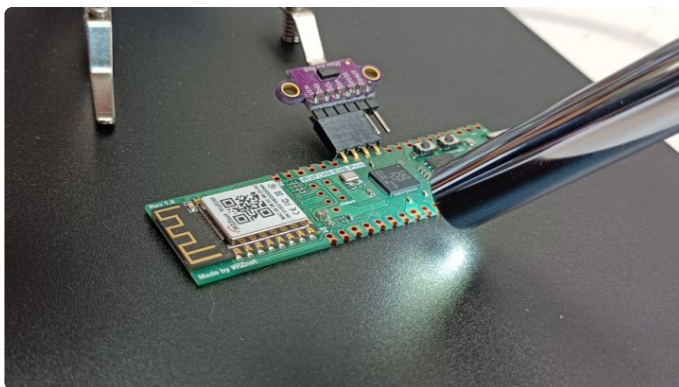
Figure 4: The endoscope with built-in LED ring lets you look at details from a different angle. It can also look inside objects.
