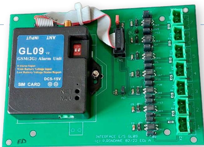
Figure 2: A closer look at the adapter PCB.
