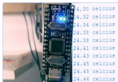
Figure 4: The Arduino Nano board used in this project, with the flow of the readings showing on the right.
