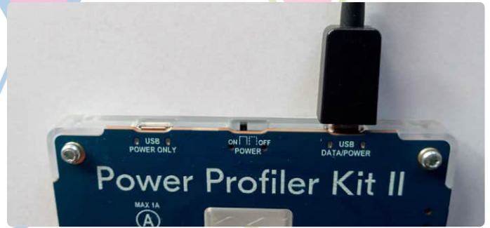
Figure 5: Connect the Power Profiler Kit II to your PC.
