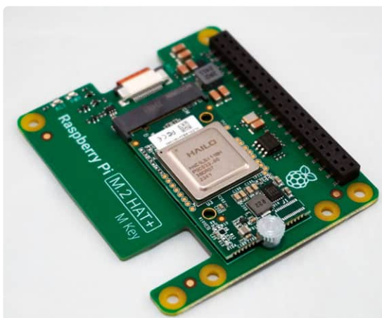
◀ Figure 2: The Kit consists of the Hailo-8L chip on its M.2-format accelerator board connected to the Raspberry Pi M.2 HAT+.
