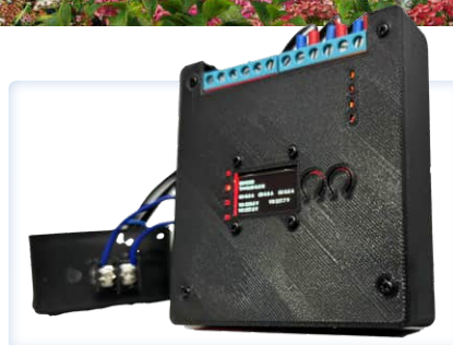
ESP32 Energy Meter Running with Home Assistant
