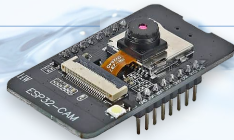
Figure 4: The ESP32-CAM is the heart of this project.
