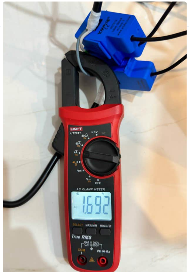
Figure 8: Clamp meter setup for calibration.
