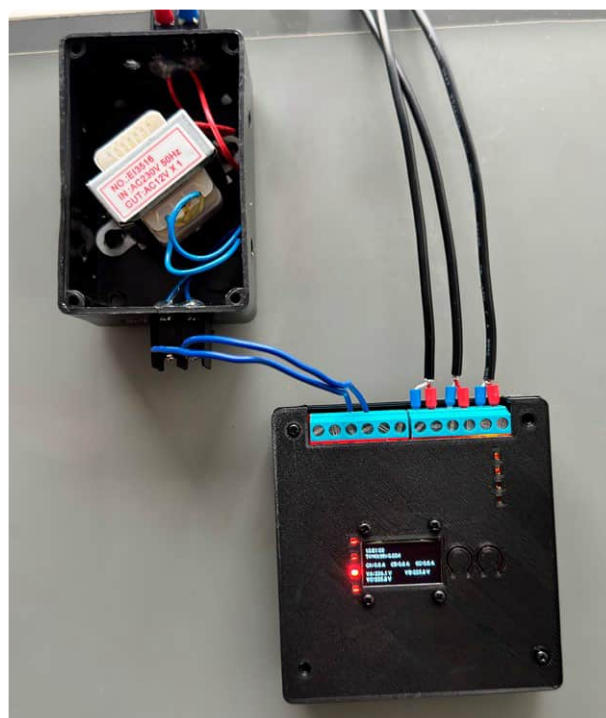
Figure 3: 220 V to 12 V Step-down transformer setup within a custom enclosure.
