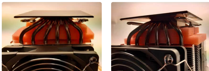
Figure 4: Copper sheet on top of the CPU cooler.
