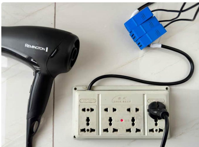
Figure 7: Setup for testing and calibrating the ESP32 Energy Meter using a variable load.
