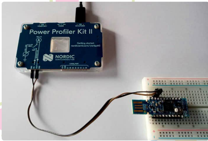
Figure 4: The Power Profiler Kit II ready to measure the current consumption of the nRF52840 Dongle in Source Meter mode.
