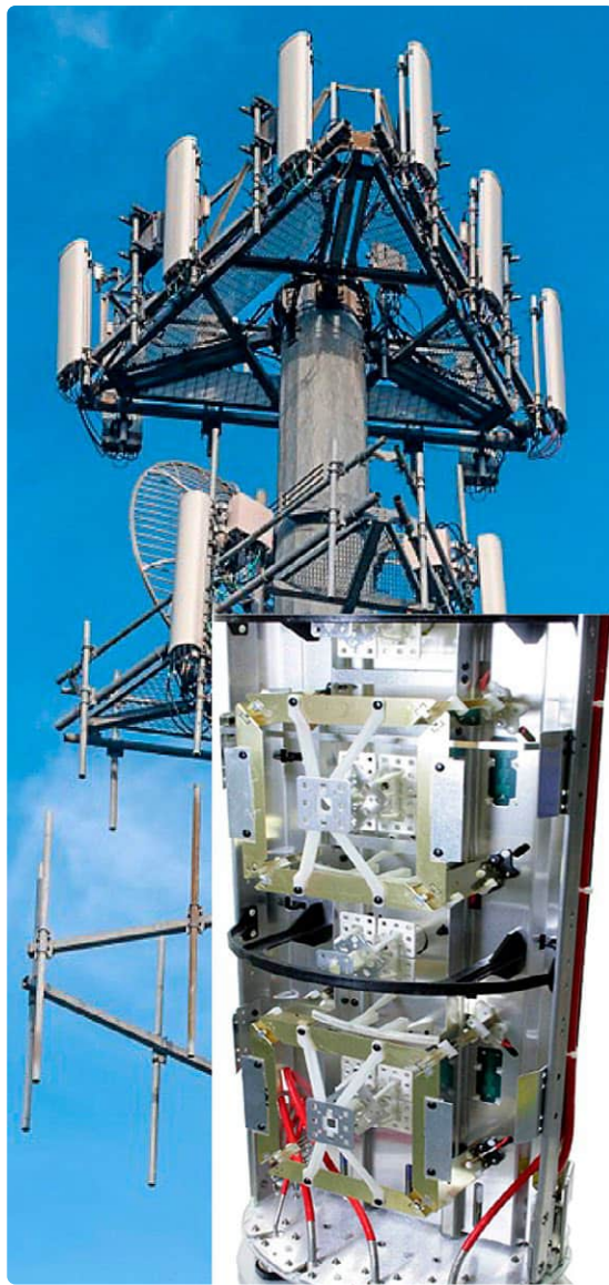
Figure 2: A typical 4G (5G) tower for 700 MHz and 1,800 MHz bands, with a detailed view of a reflector's interior.
