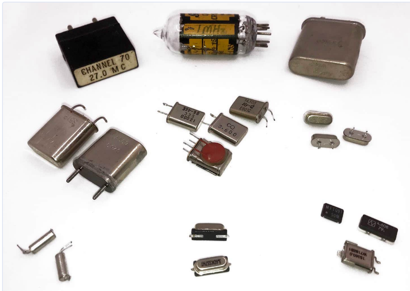
Figure 2: Various ancient and modern crystals. Top: older types. Middle (from left to right): HC6/U, HC49/U (one with a red PTC device used as an "oven") and HC49S low-profile through-hole types. Bottom (from left to right): 32,768 Hz watch crystals, HC49SMD, and other SMD types.
