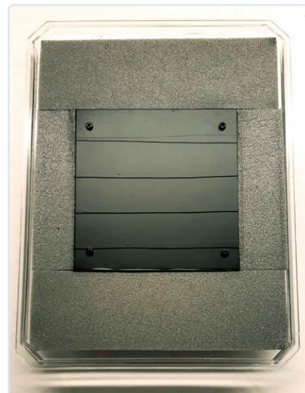
Figure 6: Black copper sheet with the sheet of acrylic around it. I covered the acrylic with some more insulation to provide a soft seal for the bell jar.
