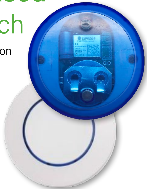
Figure 1: The ESP32-C2-based Coin Cell Switch in its enclosure.
