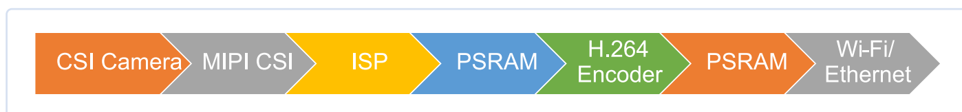
Figure 6: Example data flow for an IP camera.
