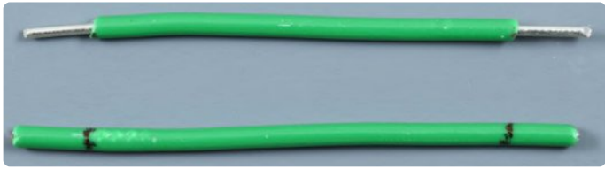
Figure 3: One wire marked and another one stripped. The remaining insulation should be 3 cm long.
