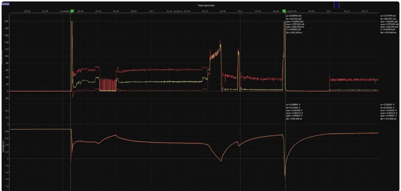
Figure 5: Scope screenshot of voltage and current values during the transmission of a standard data packet.
