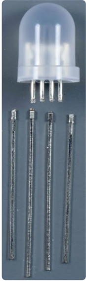
Figure 7: The leads of RGB LED WS2812D-F8 cut just above the widening.
