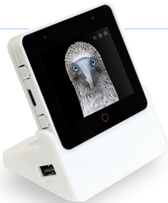
Figure 3: ESP32-S3-BOX-3 comes with a 2.4-inch display, dual microphones, and speaker.
