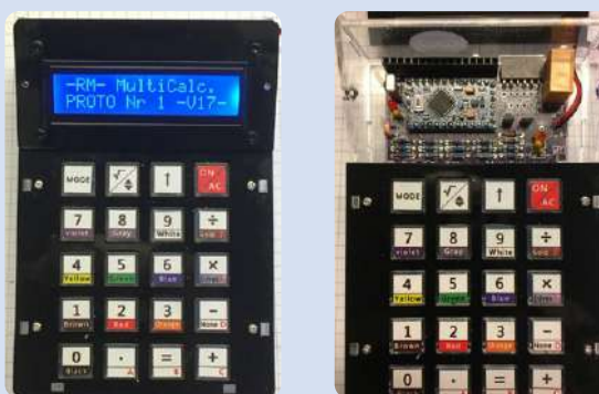
Figure 4: The Multicalculator: outside and inside.
