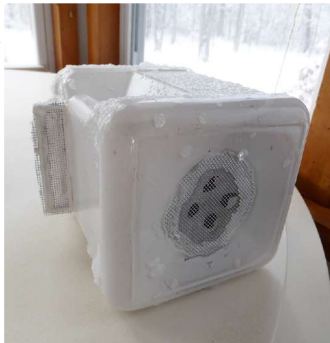
Figure 9: Sensor housing detail. All vents are screened to prevent bio instead of software bugs ;-).
