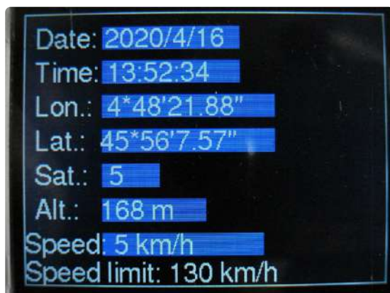
Figure 6: GPS data is available on Screen 3. This is also the screen that provides access to the speed limit definitions on Screen 4.
