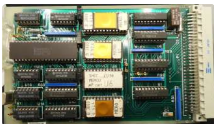
Figure 1: Dating back to the mid-1980s, this board features an 8085 microprocessor. Combined with six other boards (see article header), it became as fully featured as today's microcontrollers!
