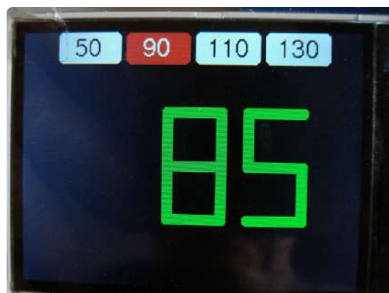
Figure 4: On Screen 2, the actual speed is presented on a simulated 7-segment display.
