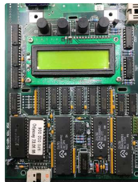
Figure 2: Another workhorse of early embedded systems was Zilog's Z80. Here it is accompanied by a serial I/O controller (SIO) and counter/timer circuit (CTC).
