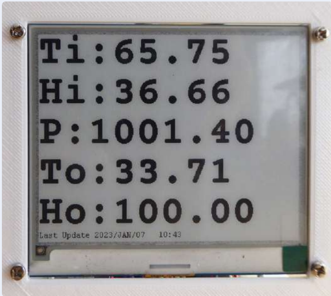
Figure 2: My ePaper display shows the temperature (in °F), relative humidity, and barometric pressure uncorrected/not normalized. The “i” and “o” subscripts refer to inside and outside. Only outside pressure is displayed.
