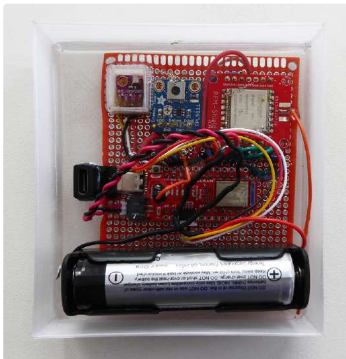
Figure 8: Sensor board embedded in epoxy. Note the small plastic square in the upper-left-hand corner that prevented the epoxy from covering the sensor. Also note the USB-C right-angle dongle (left, middle) that permits access to the board for recharging and software updates.
