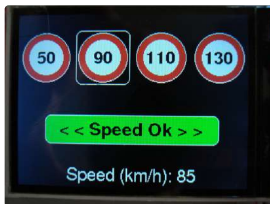
Figure 3: Screen 1 shows the speed limits as round traffic signs together with a brief message.
