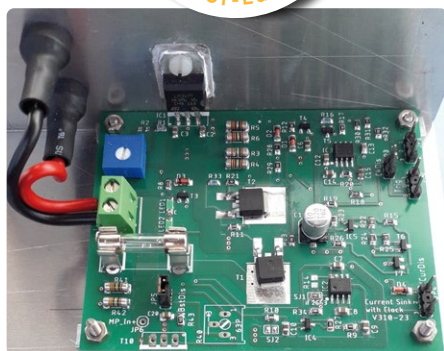
Figure 1: The current sink without the booster and with a large heatsink plate (left). The plastic screw for the LM317 was not a good idea. The fully populated board with the booster is shown on the right.
