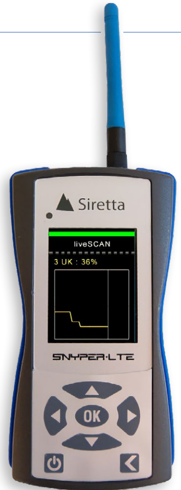
Figure 1: The SNYPER-LTE Spectrum delivers a wealth of data that eases antenna selection and optimal location for cellular wireless equipment.
