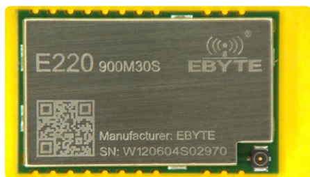
Figure 4: Modules ending in 'S' offer IPEX / U.FL antenna output.
