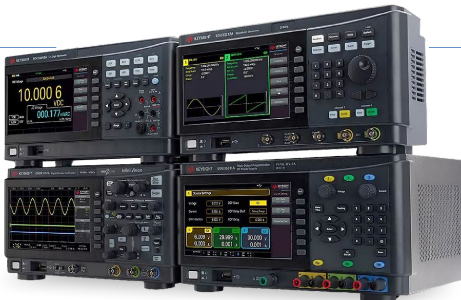
Figure 4: Designed for remote operation and collaboration, Keysight's Smart Bench Essentials test and measurement equipment unites traditional operation with cloud connectivity.
