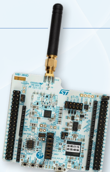
Figure 3: The NUCLEO-WL55JC is compatible with standardized as well as proprietary protocols such as LoRaWAN, Sigfox, wM-Bus and more.
