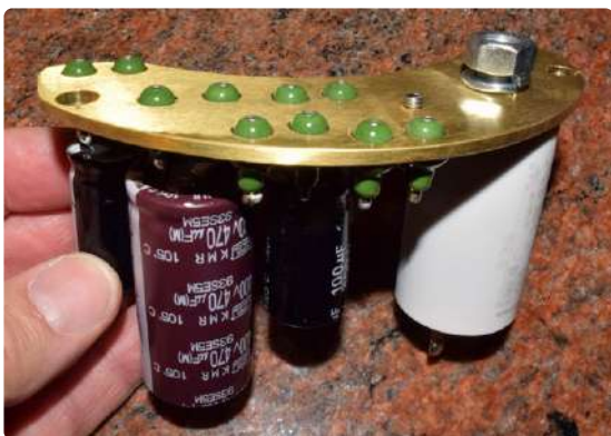
Figure 14: The bulky electrolytic capacitors need their own brass plate.
