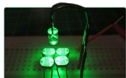
Using Light for Sound Effects: LDR-Based Voltage-Controlled 24 dB/oct Synthesizer Filter
