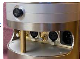
Figure 19: A recess at the rear holds the input and output connectors and the mains power connector.
