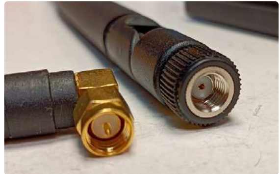
Figure 2: Antennas with SMA connectors. Left is right and right is wrong for Opera Cake and HackRF One.
