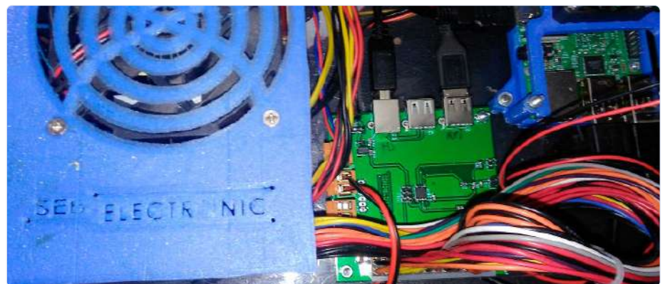
Figure 4: ATX power supply connected to the PCB.
