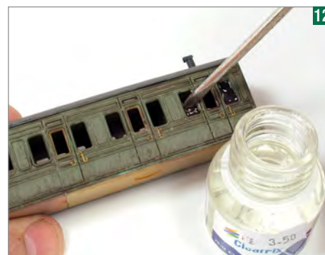
12 Using a small screwdriver, blobs of Humbrol Clearfix are worked around the edges of each window until they fill the hole. Leave the coach on its side until dry.
