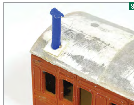
9 A chimney is made from the inner tube in a ballpoint pen. The roof canvas would be protected with cheap metal on the prototype, made from a square of plastic.
