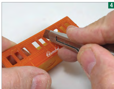
4 Both coaches are shortened by running a knife blade down the gaps beside the doors. Several careful passes are necessary to work through the plastic.
