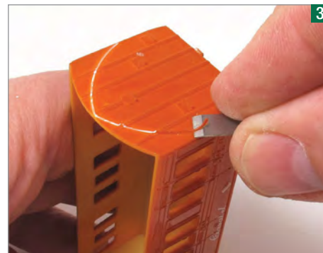
3 Handrails and steps on the body end are removed with a chisel blade. Avoid scratching the rest of the surface. A little damage will look like wear and tear.
