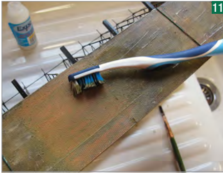
Expo tools paint stripper is safe for use on plastics and isn't drawn by capillary action. The old paint lifts after 10 minutes exposure and a little scrubbing.
