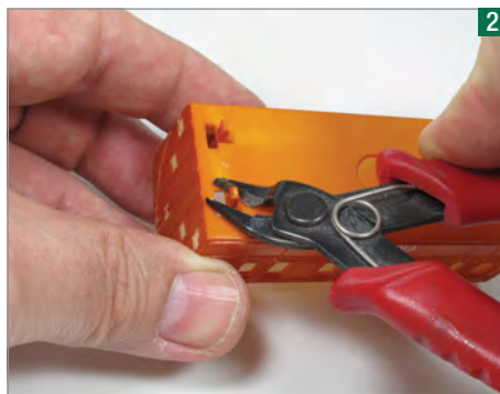
2 With the body easily removed, clips under the body that didn't break when removing the chassis are cut and removed with flush wire cutters.
