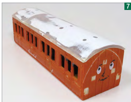
7 Cut the clear glazing from the roof with a fine saw. Sand the vents and rainstrips then fit both roof mouldings, staggering the joint with the sides.
