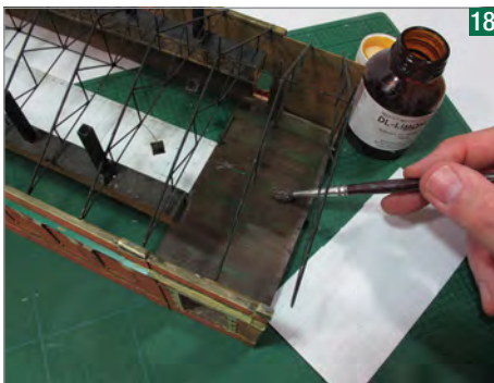
Thin plastic can't be laminated with normal solvent as it'll buckle and warp. Limonene from Wizard Models is a much gentler solvent and won't damage the plastic.
