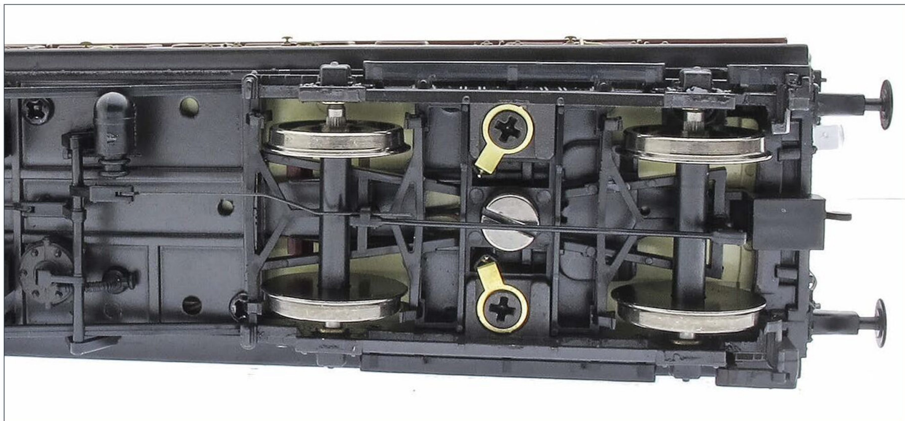
Detailed diecast bogies include current collection for the interior lighting.
