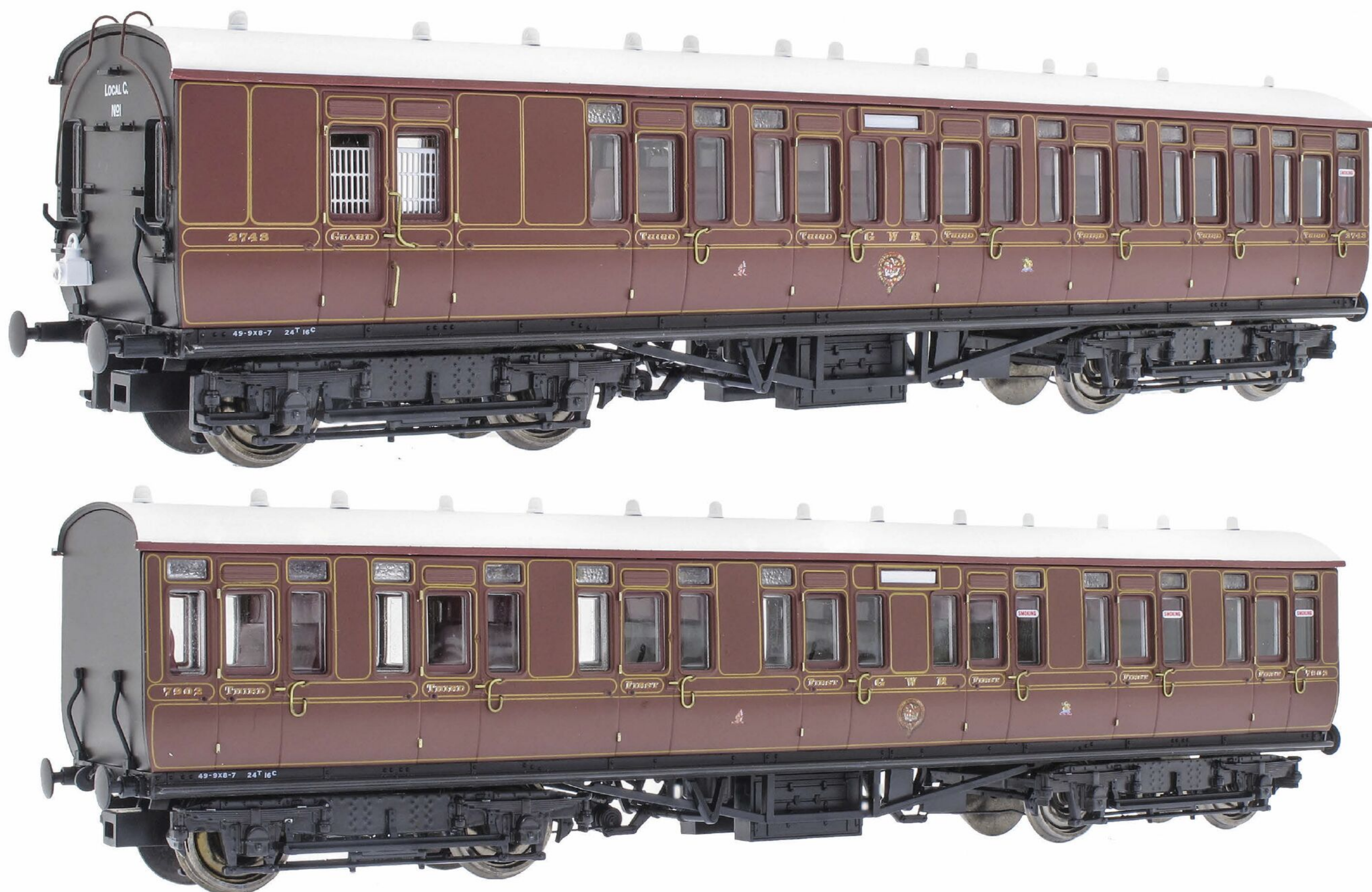
The brake end has separately-fitted communications conduits in addition to a fixed working taillamp.
