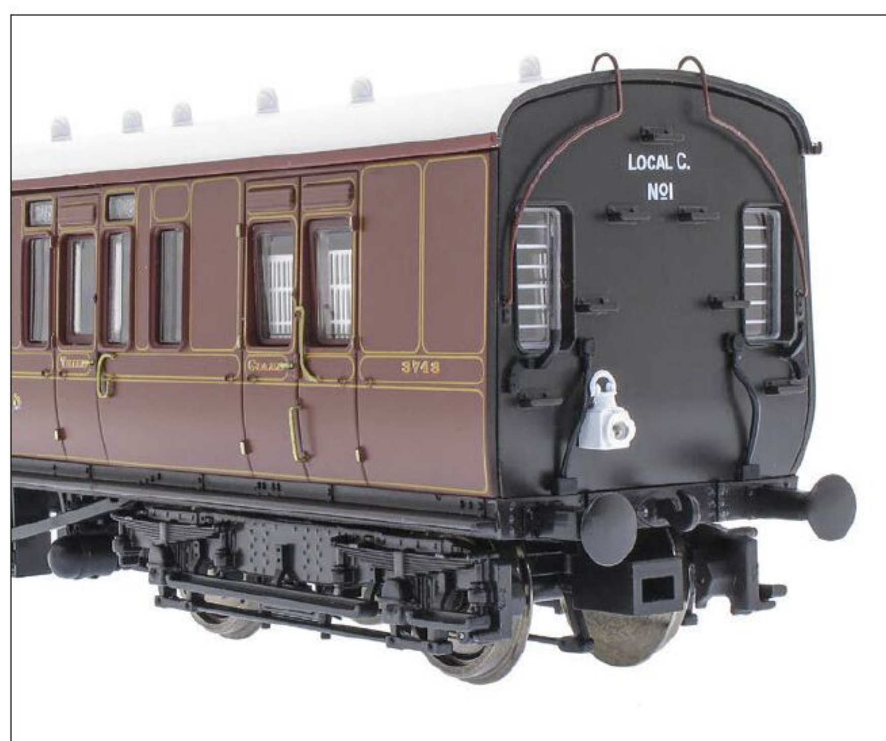
The brake end has separately-fitted communications conduits in addition to a fixed working taillamp.
