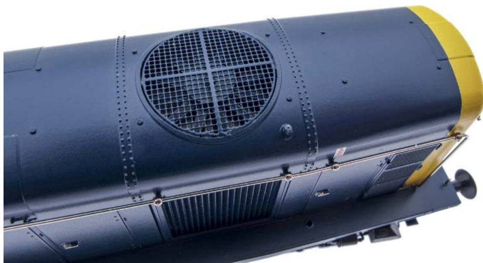
The etched fan grille is finer, giving a clear view of the fan blades.
