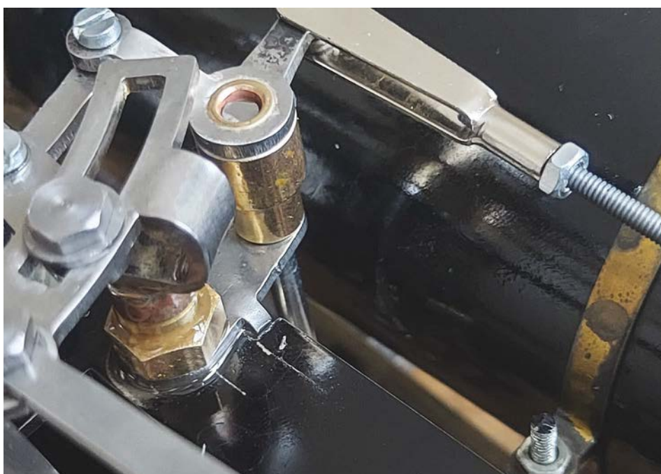
Positioning of the expansion link.
