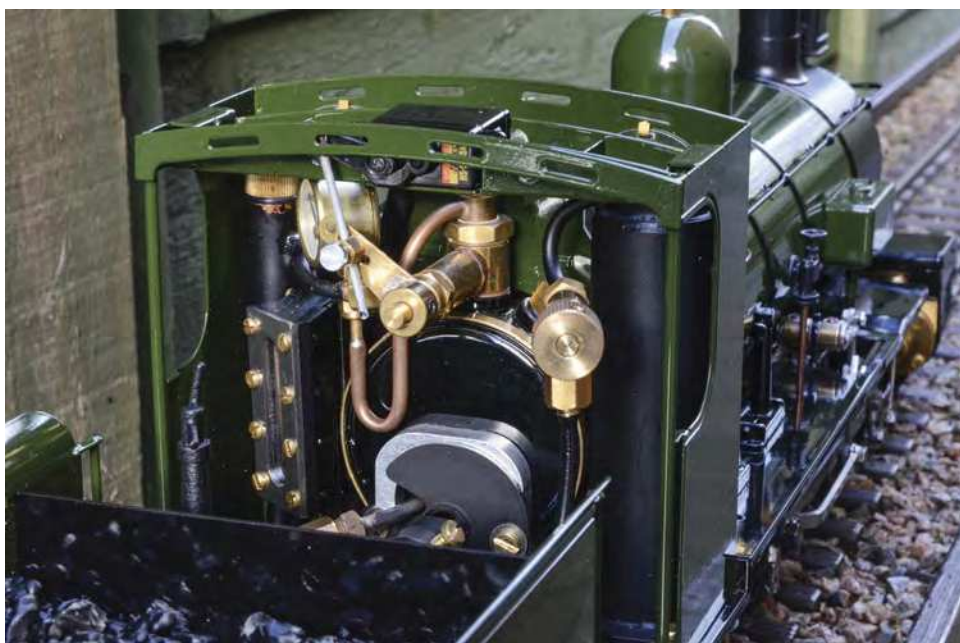
Roof removed to show the regulator servo – the controls are otherwise standard Roundhouse.
