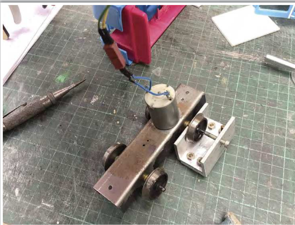
IP Chassis having its wheels removed to fit new gears and Delrin Chain for 4w drive.
