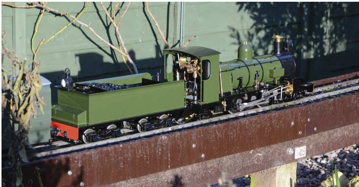
It's a long old tender! Note the colour coding on the R/C connector, which looks like it's trailing on the rail, but really isn't.
