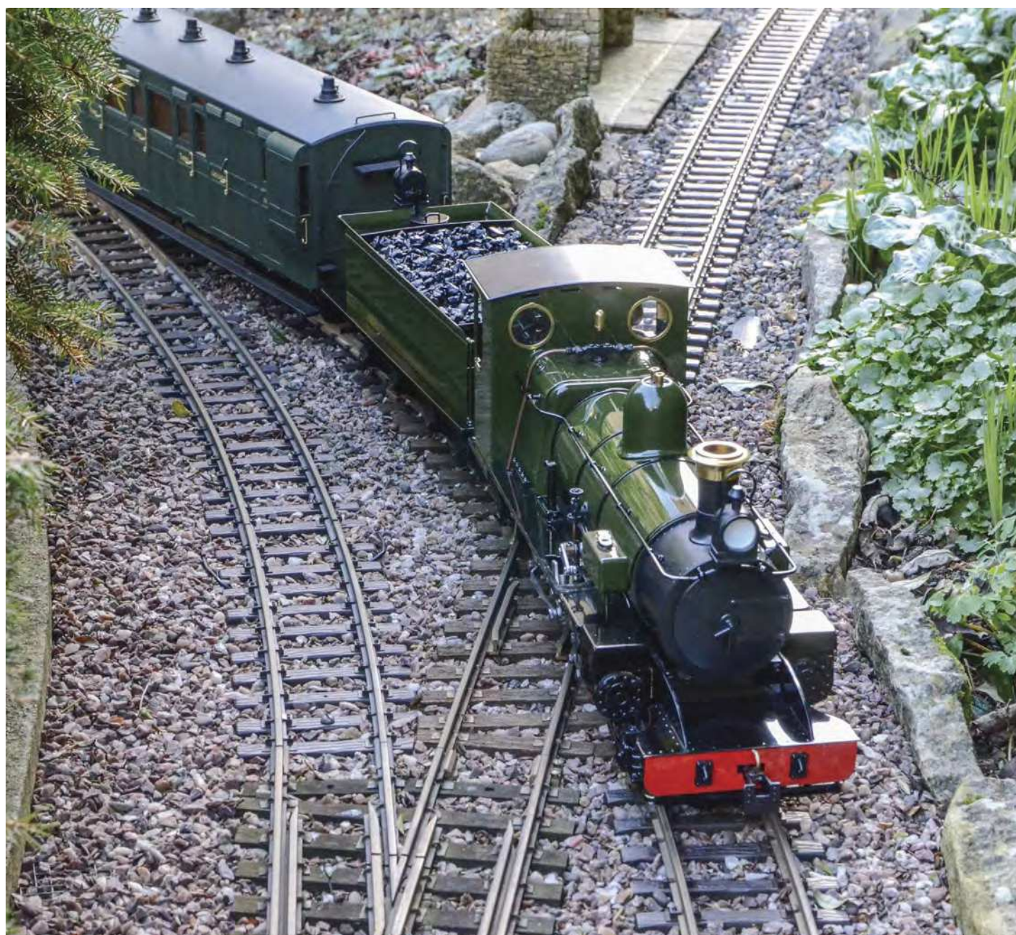
Taking the line down the 1 in 50 – the diamond crossing was scratch-built specifically for this formation.
