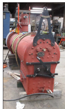
Right: The boiler hydraulic test was conducted with the unit out of the frames. Photo: Alan Keef Ltd
