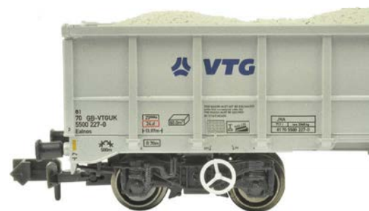
Underframe arrangement changes are most obvious from the outside, with the location of the handbrake wheel located either to the wagon centre (above), or bogie (below).
