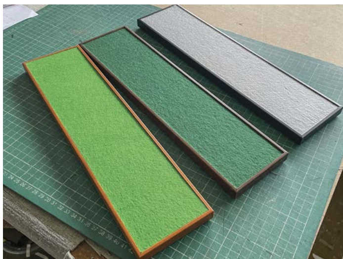
The base starts as a series of carefully-cut wooden mouldings, into which a felt-covered board is fitted.
