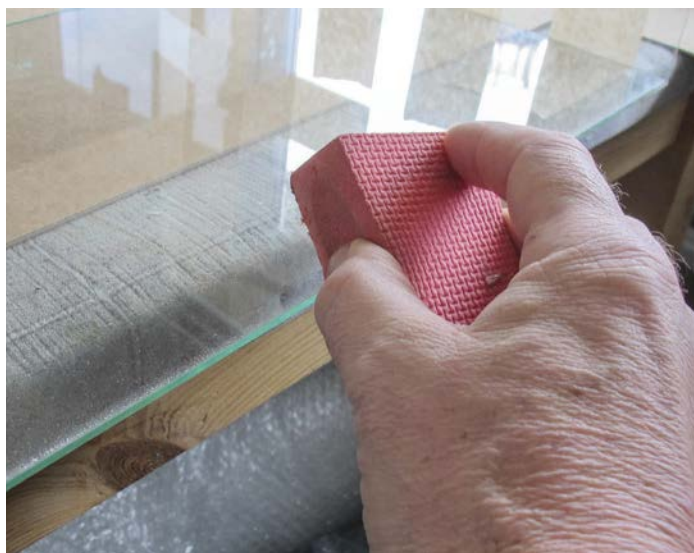
A vital step is to use a diamond sanding block to clean up the sharp glass edges.
