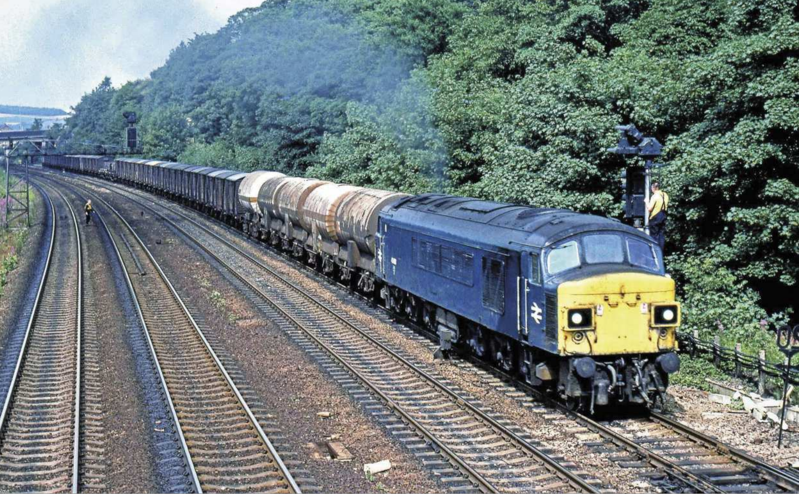
Thursday 28th July 1977: With an eruption of exhaust, 45021 heads south near Chesterfield with a traditional mixed wagonload freight formed mainly of short wheelbase vans. There are also two bogie bolster wagons of steel and five carbon dioxide tanks at the head of the consist, possibly from Haverton Hill to Coleshill. The CO2 tanks are in typically filthy condition. The service is thought to be 7M72, the 17:15 SSuX Tinsley to Bescot (arr. 20:10), which had previously run as 7O70 to Eastleigh. It will reach Bescot by way of the former South Staffs route from Wichnor Junction via Lichfield and Walsall (see article in TRACTION 233 & 234). JOHN WOOLLEY.
