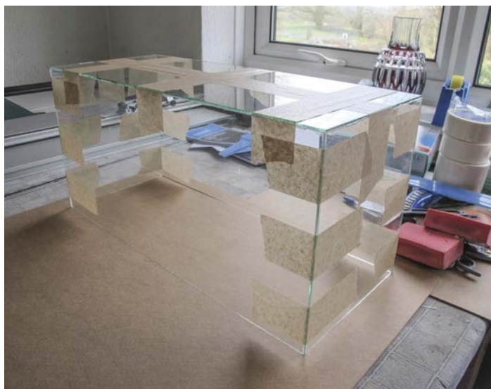
All cases are cut from 3mm thick glass, glued together with tape holding the panes in position. The adhesive is left to set overnight.
