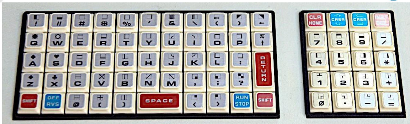
Fig. 5 - The small keyboard with rubber keys of the early PETs (photo: Soupmeister - source: Wikimedia Commons)
