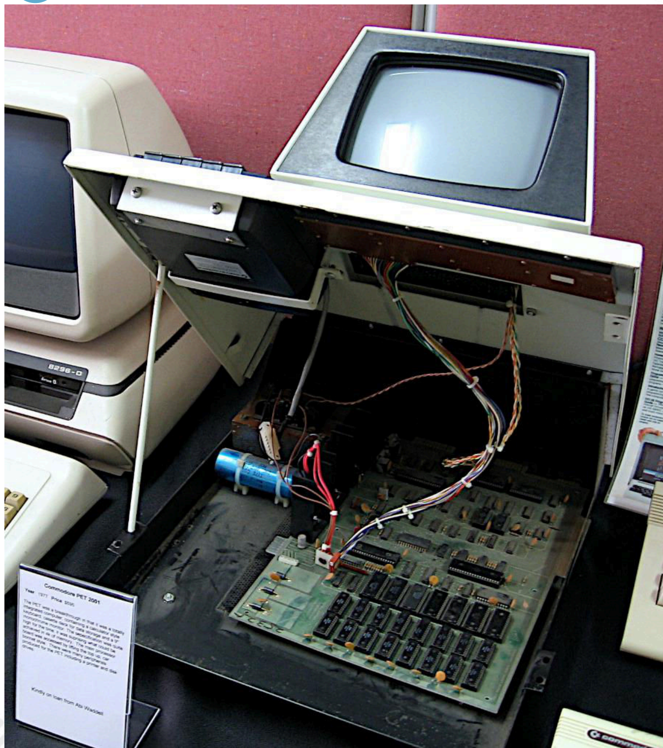
Fig. 4 - The "car hood" opening of the PET (photo: Marcin Wichary - source: Wikimedia Commons)
