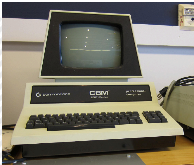
Fig. 6 - A 2001 CMB with the new keyboard and 12" monitor (photo: Jeff Keyzer)
