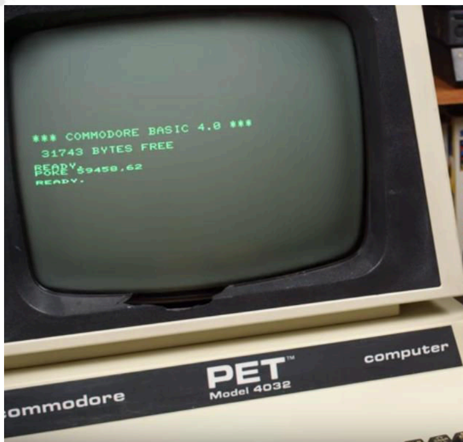
Fig. 7 - The effects of the "killer POKE", you can see the distortion on the image being compressed towards the center (photo: André Fachat - source: 6502.org)
