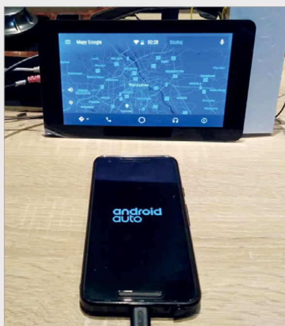
Above OpenAuto is an Android Auto emulator, allowing your Android smartphone to 'project' its interface onto your car's screen
