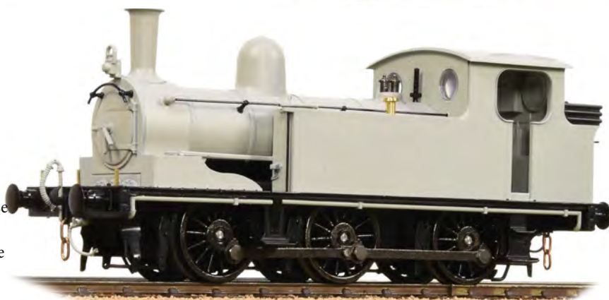
Above, Bachmann's LNER J72 0-6-0, one of four tooling variants. Note the three-link couplings and headlamp.
