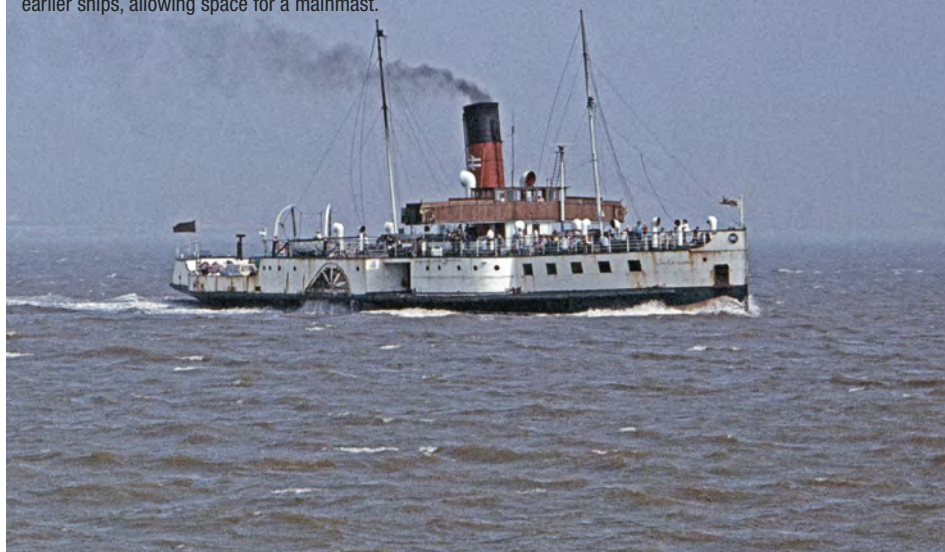
PS Lincoln Castle heads for New Holland with a full complement of passengers and cars. Note the position of her bridge deck and funnel being further forward to that of the earlier ships, allowing space for a mainmast.
