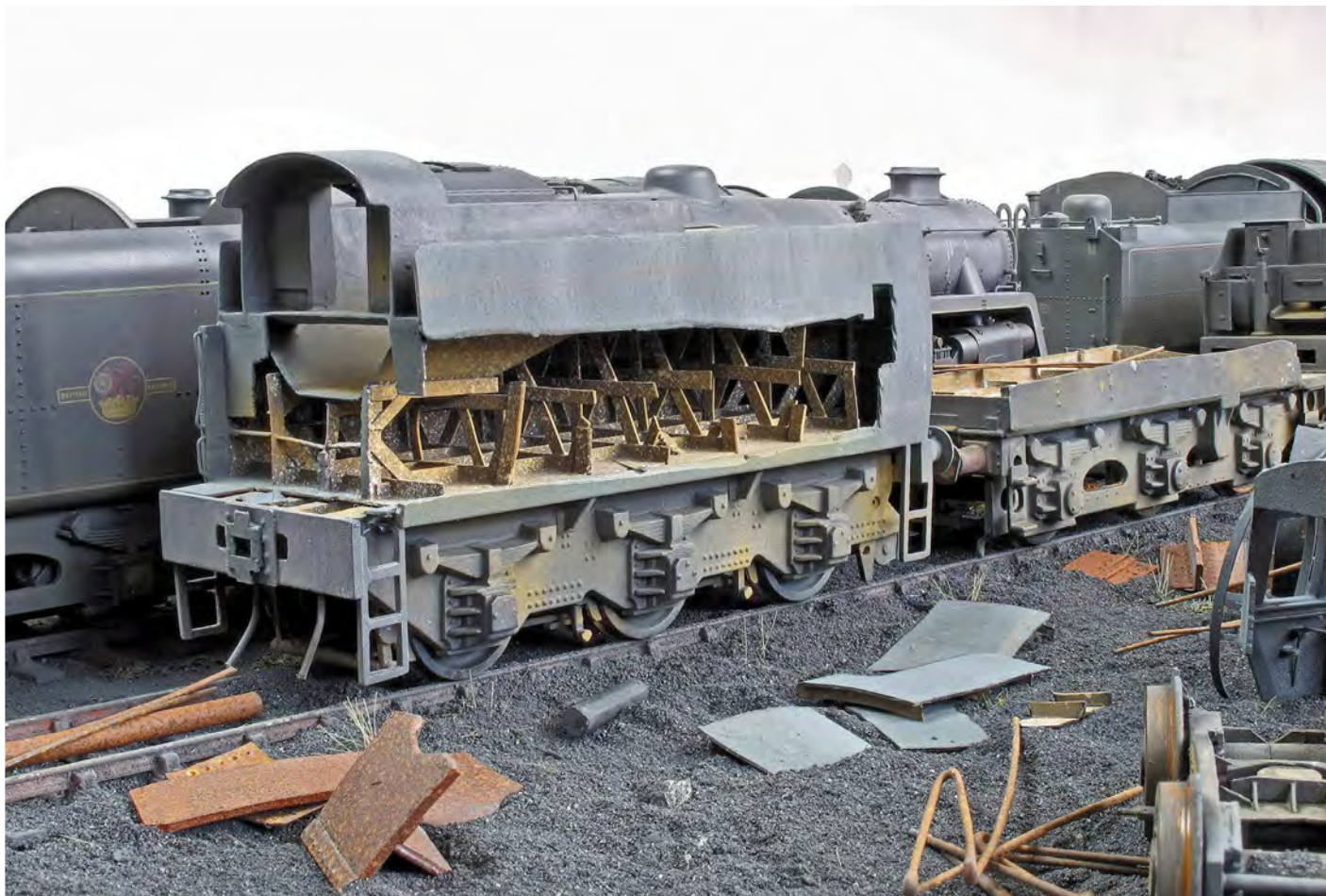
A partially dismembered Bulleid tender reveals its secrets of construction. The inner struts are designed to strengthen the tank and also to prevent surging. You can see a sectioned Bulleid tender in real life in the National Railway Museum.
