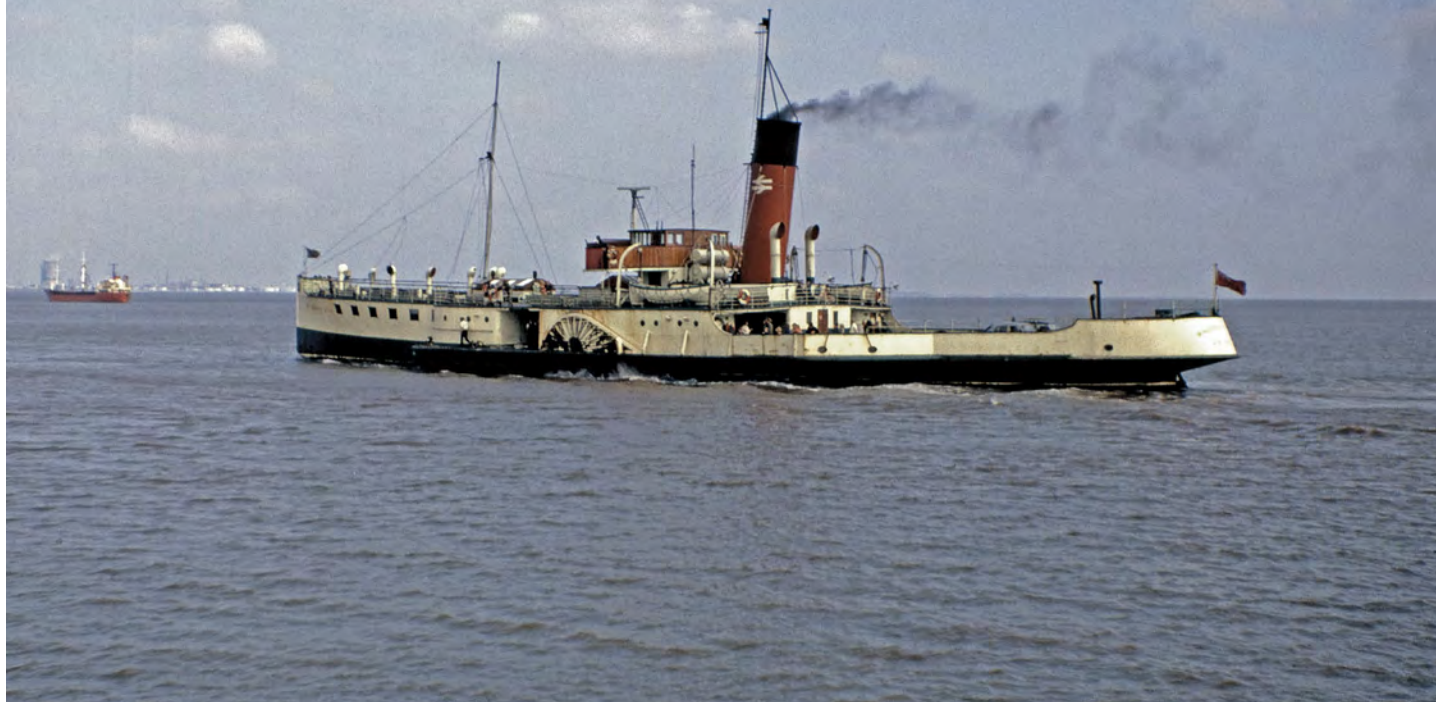
PS Lincoln Castle heads for New Holland with a full complement of passengers and cars. Note the position of her bridge deck and funnel being further forward to that of the earlier ships, allowing space for a mainmast.
