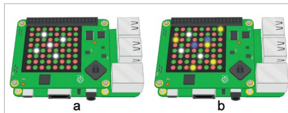
Figure 4 The incomplete puzzle in Figure 4a can be solved by moving the cursor under one of the queens and pressing the joystick button. The white queens in Figure 4b were placed correctly, the blue queens were in the wrong place, and the yellow queens are the ones you needed to place in order to complete the puzzle
