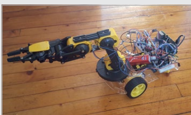
Above Ahmed first experimented with mounting the arm on a two-wheeled chassis, before opting to customise an OWI All Terrain Robot kit
