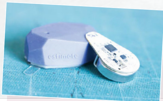
Left A beacon is attached to Bean's collar, and three Raspberry Pi devices are used to triangulate the dog's position
