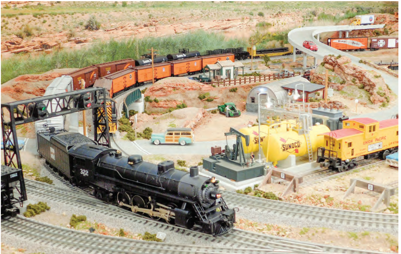
Outer loop curvature is 072 and the inner loop is 060 minimum diameter. A Mikado approaches the outer loop with its long consist.
