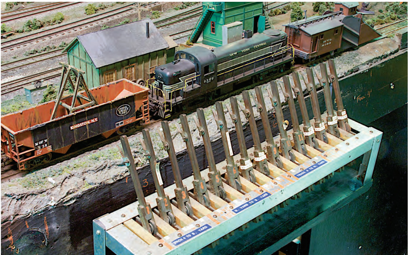
A well-engineered switch control panel with realistic armstrong levers was built in the early days of the club and is still in use.
