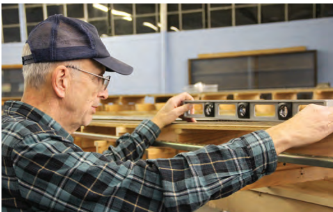
Grades are kept to a maximum 1 percent change in elevation.
