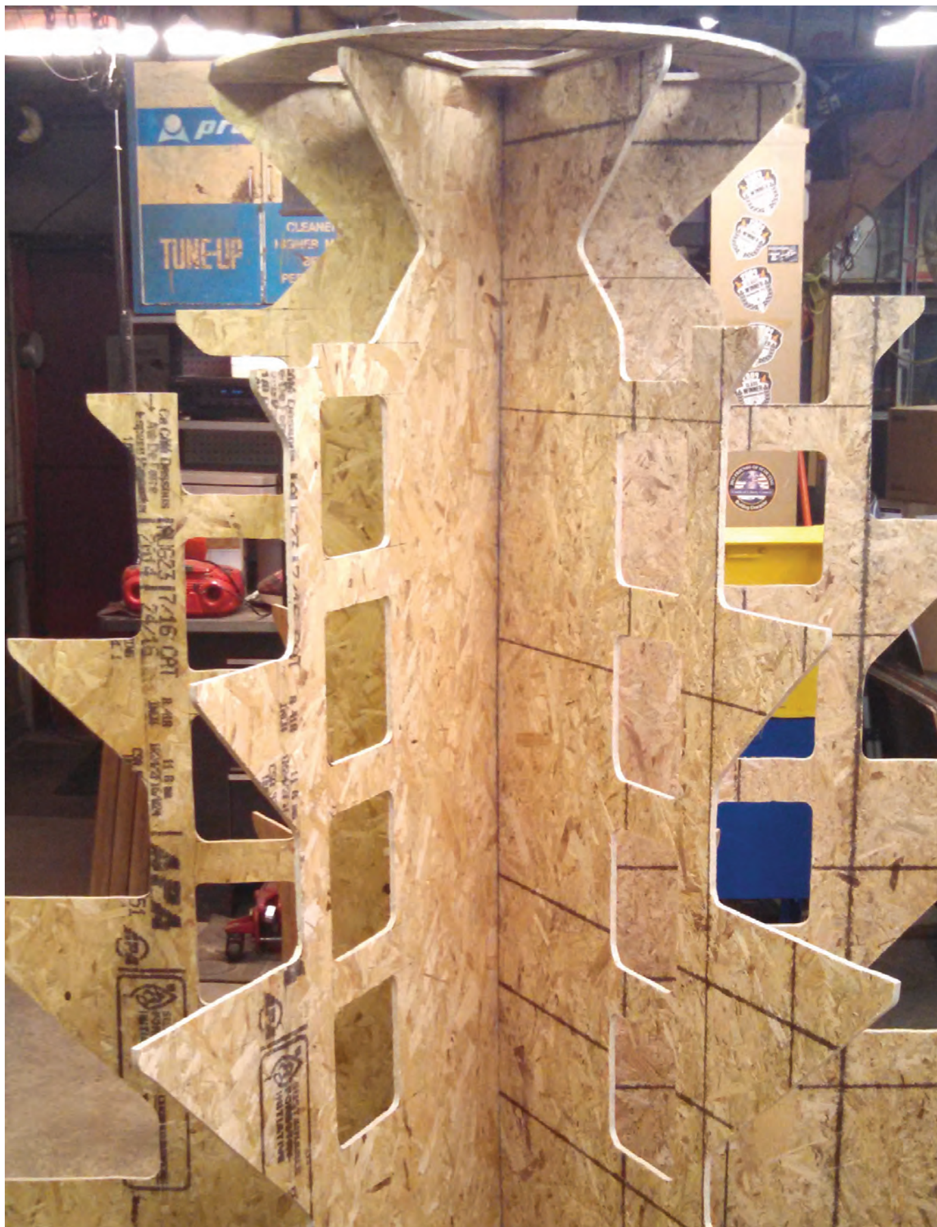
Six vertical sections of plywood make up the primary supporting structure.
