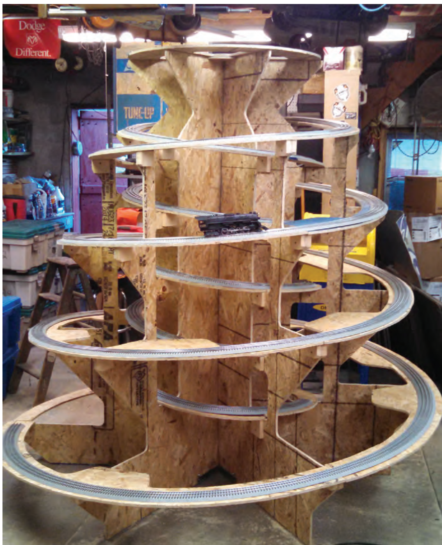
With track in place, a lone Lionel Polar Express Berkshire sans tender and cars are used to conduct a test run.
