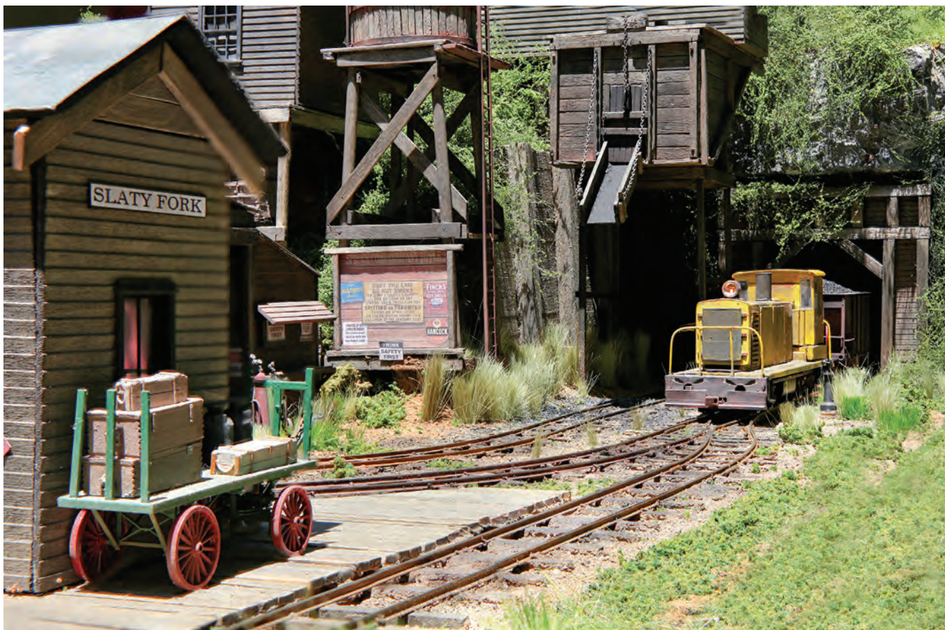
The "Yellow Dog" way freight exits the North End Hickory tunnel as it approaches Slaty Fork station. Diesel No. 27 was constructed from the base of an HO scale Bachmann GP9 and features a SoundTraxx Tsunami EMD 567 sound decoder along with a rectangular speaker mounted in the body.
