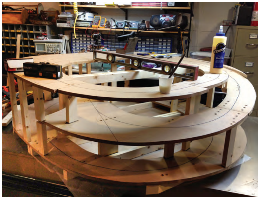
Risers were added to the multiple levels, and the interchange grade was formed.
