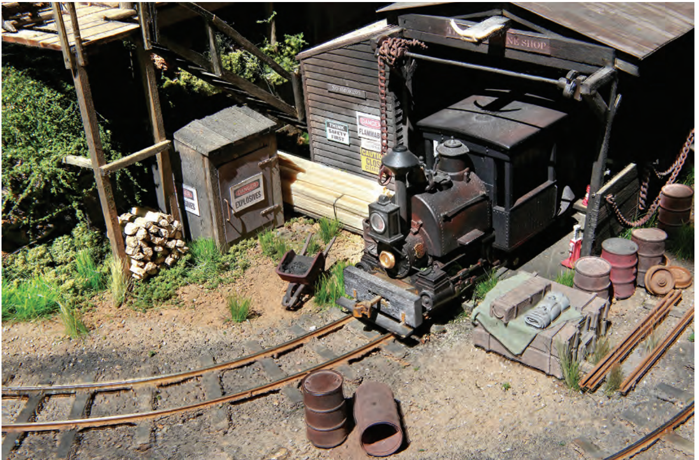
Ol' No. 1 sits in the locomotive service shed at Spruce Coal Company awaiting a fresh crew. Like Porter No. 2, ol' No. 1 started as a Bachmann 0-4-2 shortened and with trailing wheels removed to make it a 0-4-0. The tender was scratchbuilt from an HO gondola and uses an On30 passenger truck. For reliability, all wheels are fitted for electrical pickup.
