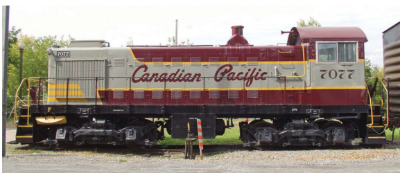
Both of Canada's major railroads, CN and CP Rail, are well represented at Exporail along with many of the nation's smaller carriers. CP Rail No. 7077 is an S2 switcher.
