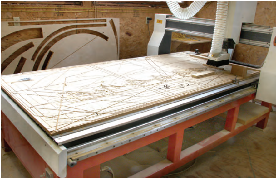
Another tool in the Dunham Studios computer-age arsenal is this 4' x 8' computer-driven CNC router.
