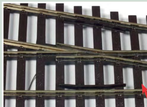
The completely metal live frog point.
