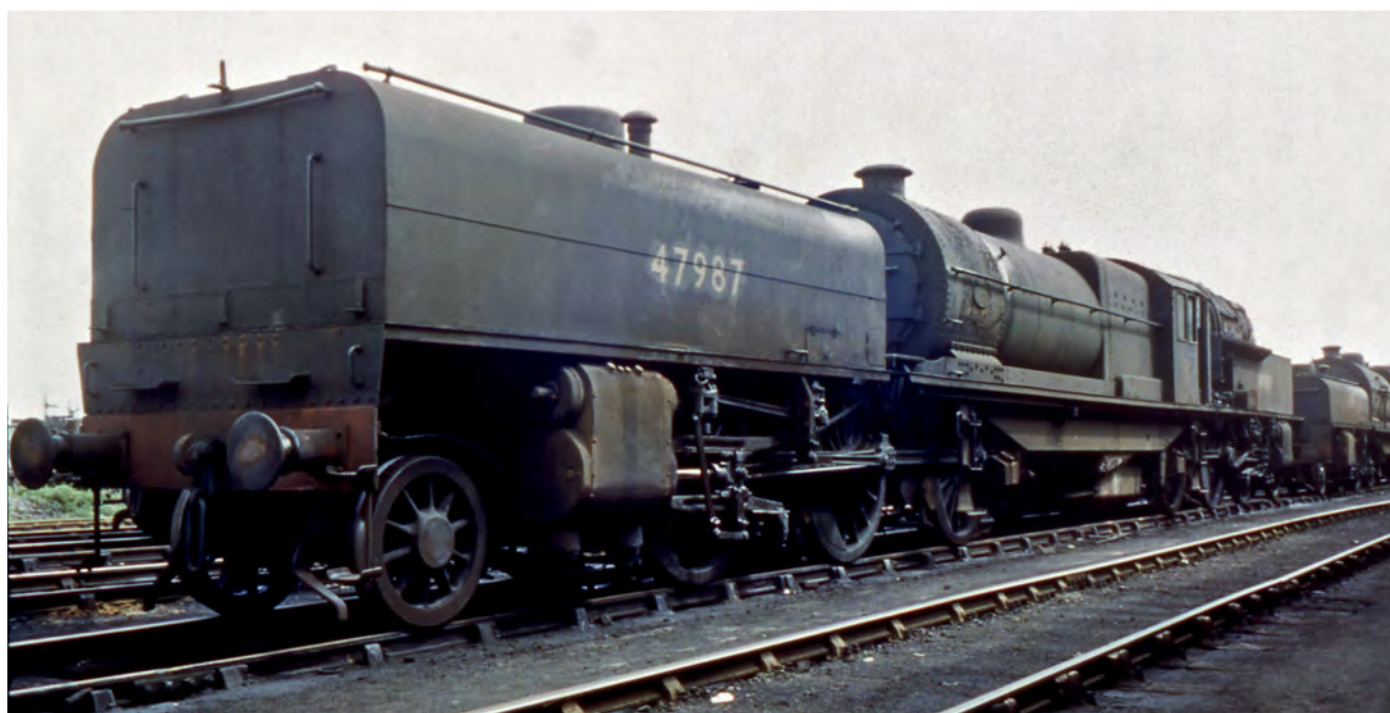
No. 47987 stabled at Toton on June 23, 1956 is an ideal example for modellers wanting to weather and super-detail their BR 'Garratt'. The Hasland-based locomotive is less than a year away from withdrawal. Behind is No. 47998, one of the three prototypes, identifiable by its smaller water tanks. T OWEN/COLOUR-RAIL.COM BRM2710
