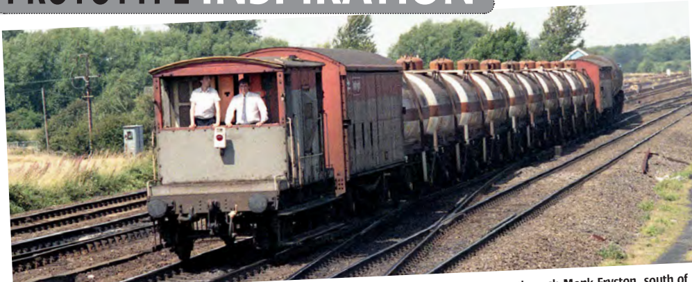
A Railfreight red/grey CAR brake van attached to the rear of a rake of ICI tank wagons passes through Monk Fryston, south of York, on July 30 1992. Note the battery powered tail light attached to the rear of the van. 53A MODELS /JOHN TURNER
