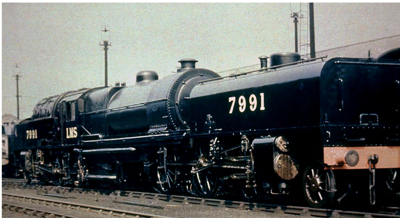
Fresh from the Crewe Works paint shop, No. 7991 shows off its LMS paintwork and rotary bunker in 1938. H M LANE/COLOUR-RAIL.COM LM111
