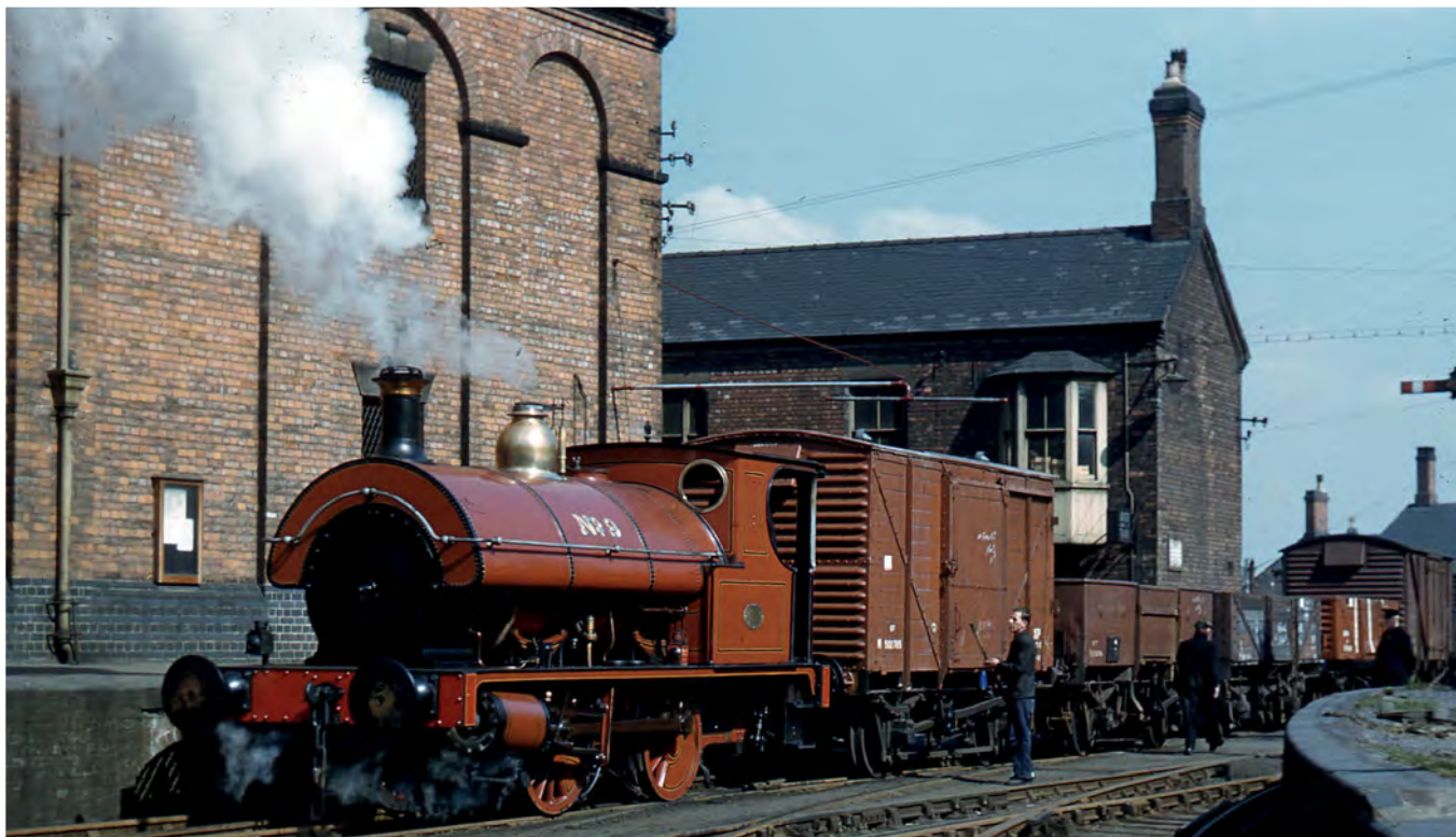
Immaculate in red with gleaming brass safety valve bonnet, Bass 0-4-0ST No. 9 shunts a typical cut of wagons under the watchful eye of the shunter and an inspector. Behind the 1901-built tank are an ex-LMS 12t vent van, ex-LNER 13t 'High', a five-plank open, an ex-works shock absorbing open wagon and a BR 12t vent van. By the early-1960s around 50% of wagons used to deliver beer were of the shock absorbing type. COLOUR-RAIL.COM 112593
