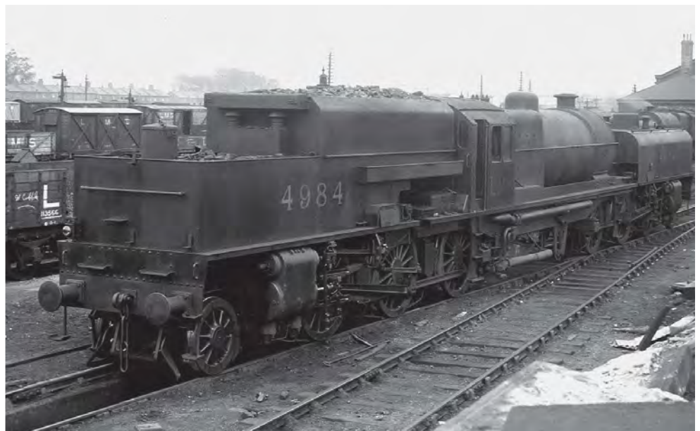
A rear view of No. 4984 in original condition showing the lengthy coal bunker, fire iron trough and a host of original 1930s details, as seen on Hattons' new model. RAIL ARCHIVE STEPHENSON
