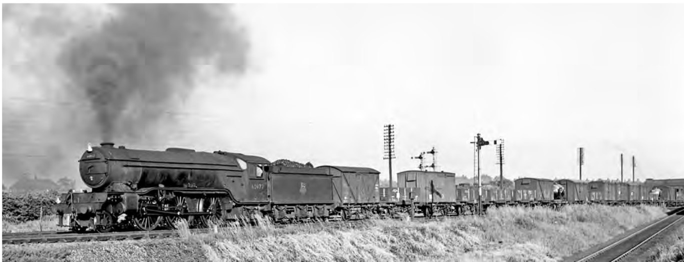
By the early-1960s around 50% of wagons used to deliver beer were of the shock absorbing type, much in evidence in this 1948 view of 'V2' 2-6-2 No. 60977 joining the former Great Central London Extension at Bulwell Common, near Nottingham, with an evening Burton-York beer train. As well as numerous shock absorbing opens (identified by the white vertical stripes), the train includes 12t vent vans of various origins and flat wagons loaded with road-going tank trailers. T.G. HEPBURN/RAIL ARCHIVE STEPHENSON
