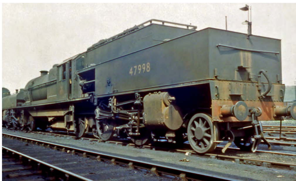
No.47998 retained its original fixed bunker until withdrawal in September 1956, although an additional coal rail was added in the 1930s. In BR black with the early emblem (no Garratt ever received the late crest), the 1927-built machine stands cold at Toton on June 23, 1956. T OWEN/COLOUR-RAIL.COM BRM2711
