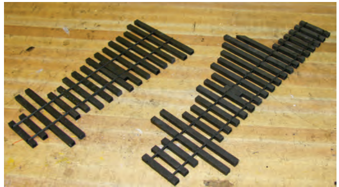
The finished tie base has been dyed black and is ready for its rails.
