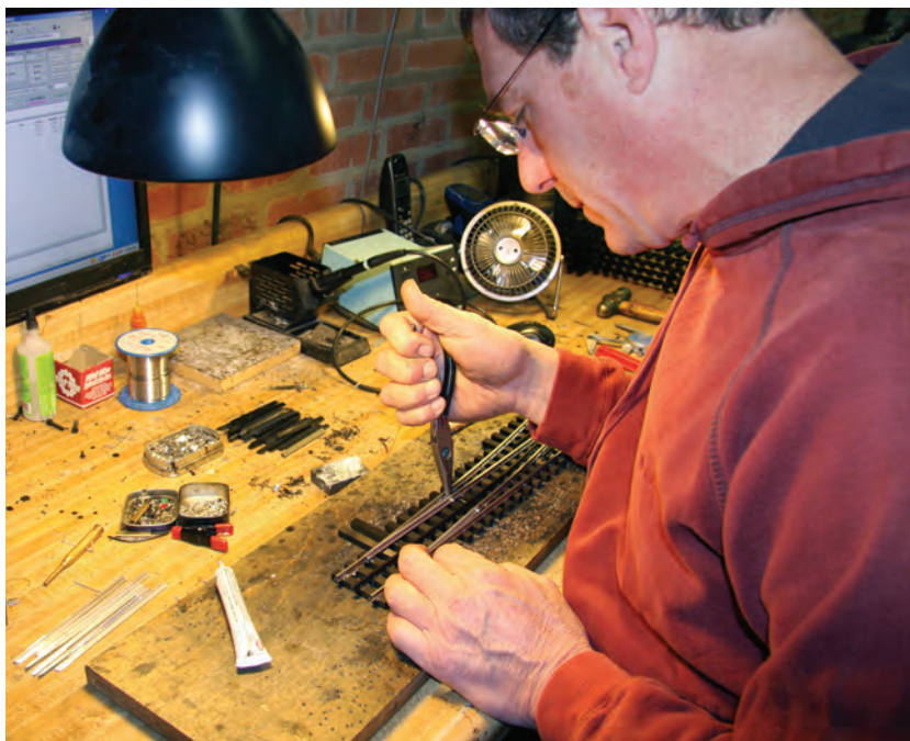
Trey Hartung begins spiking the movable point rails to their pivot points on the ties.
