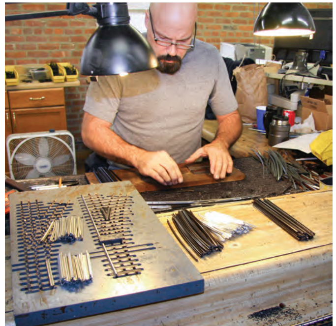
Chad Muehlbauer begins bending rails to specific angles for each switch. The dye for spiking the rails to the ties is just to his right.
