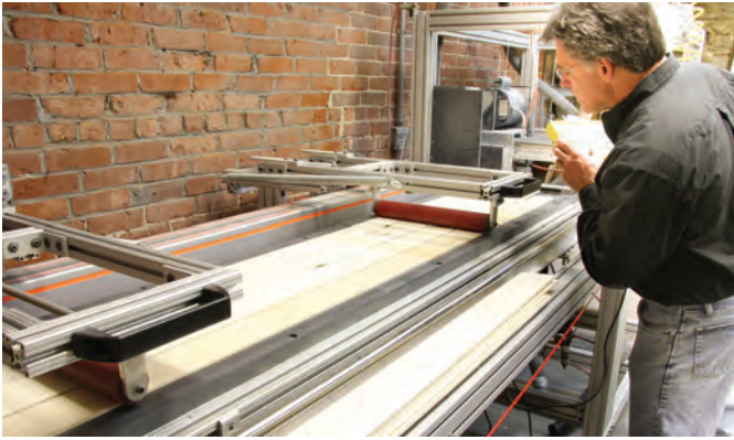
Steve prepares machined slats of aspen for processing into ties. The slats are cut into the correct widths for the ties of various sizes.
