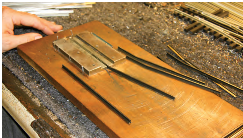
Each black center rail is bent to its exact angle needed for the switch.
