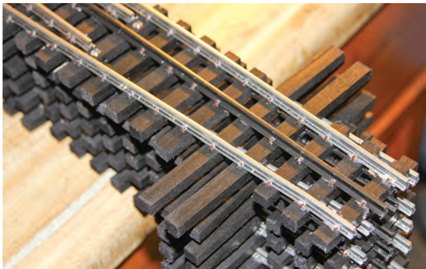
The basic switch assembly now awaits the movable point rails and the throw bar.
