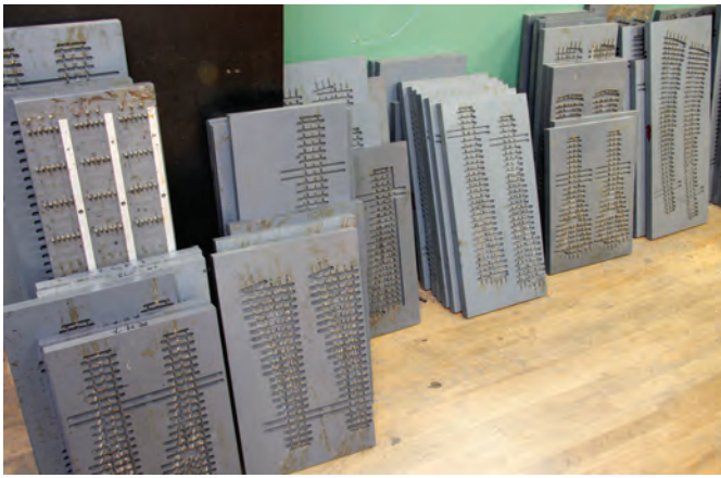
Carefully machined tooling for each switch awaits the building process.
