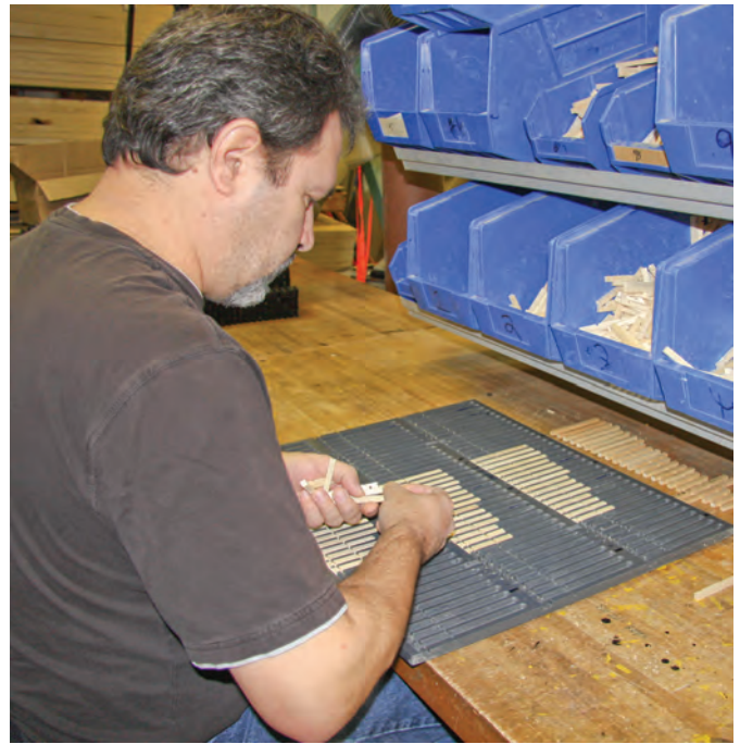
Keith Gencarelli positions the ties carefully into the tooling base. The ties are placed into the base with the bottom side up.
