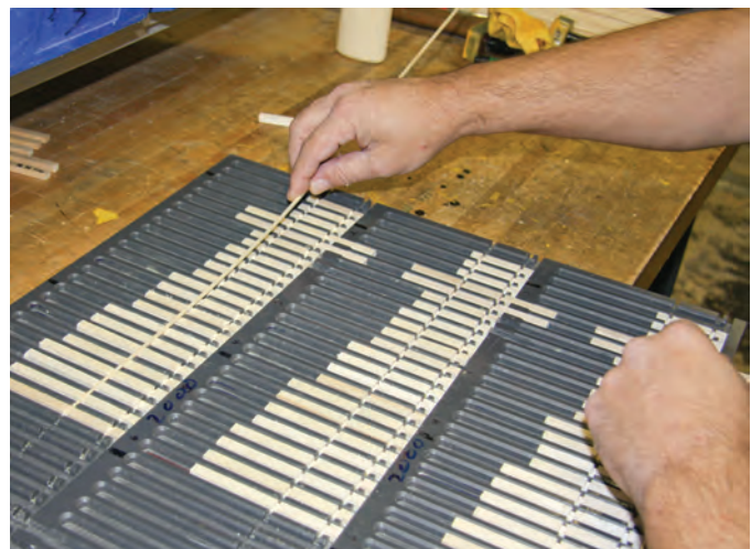
...and the wooden stringer is added into the tie base and trimmed to length.
