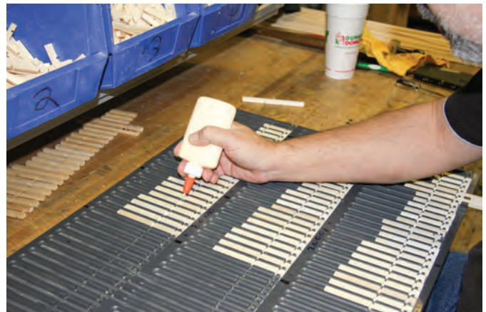
A drop of glue is added to each carefully machined slot in the ties...
