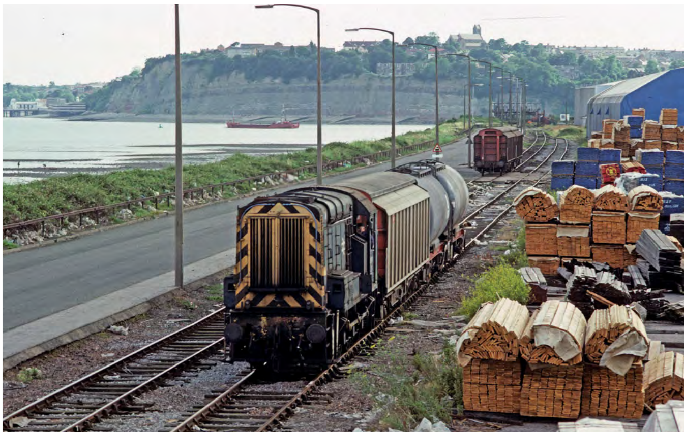
South and west of the extensive Tidal Sidings yard was a complex network of lines in Cardiff docks. In 1988, 08 796 leaves the last siding in the complex. In the background is Penarth, on the other side of the Taff estuary. Behind the 08 is a VGA van and two TTA fuel tanks (produced by Bachmann/Farish in N and OO) from Currans oil terminal deep in the docks. The VGA wagon is loaded with imported timber from Scandinavia.
