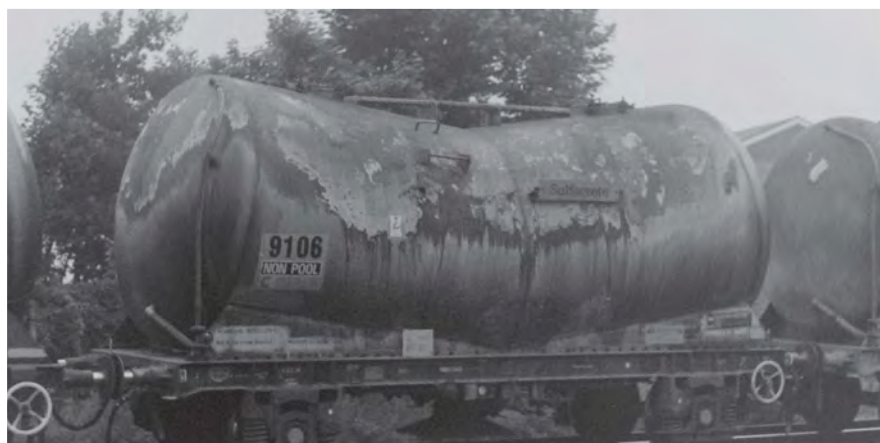
APCM9106: Another heavily-weathered wagon is this example of the later single 'Chevron' type with Gloucester floating-pedestal suspension seen at Nunhead in August 1981. The brake gear was upgraded, air brakes replacing vacuum, which did away with the cumbersome equipment beneath the tank. Blue Circle rather gave up on the idea of nameplates and symbols because they could not be kept clean. Small commodity plates were added for special cements and this example has SULFACRETE in red on yellow. Originally produced by Lima in OO gauge, the PDA has more recently been released by Hornby in various liveries and is offered by Graham Farish in N.
