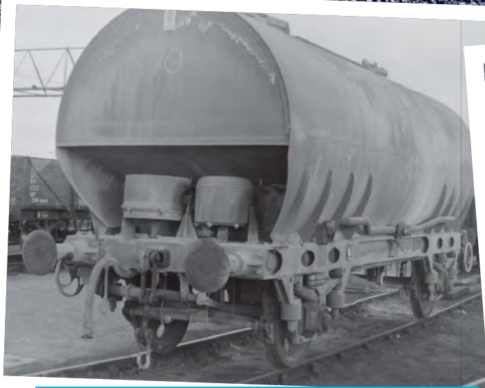
LA223: As well as the differences between the two LA batches mentioned in the text, this wagon has a different suspension. Modifications were made after the Thirsk derailment and this may not be the original. Tri-ang/Hornby produced a OO gauge model of this type from 1966 until the mid-1970s and it can still be obtained second hand at reasonable prices.
