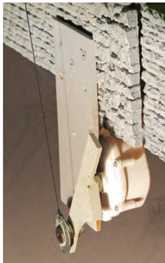
This animated Christmas deer motor has been removed from its lighted holiday host. I have found this to be an excellent, strong, quiet, and cool-running motor, which is easy to modify for continuous operating accessories.
