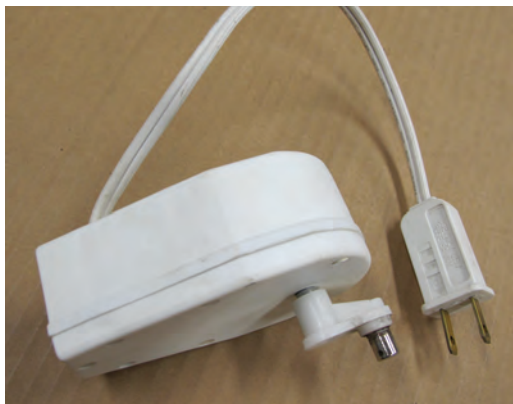
This animated Christmas deer motor has been removed from its lighted holiday host. I have found this to be an excellent, strong, quiet, and cool-running motor, which is easy to modify for continuous operating accessories.
