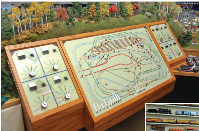
ABOVE: The main control panel provides a full schematic of the three-level, five-loop track plan.
