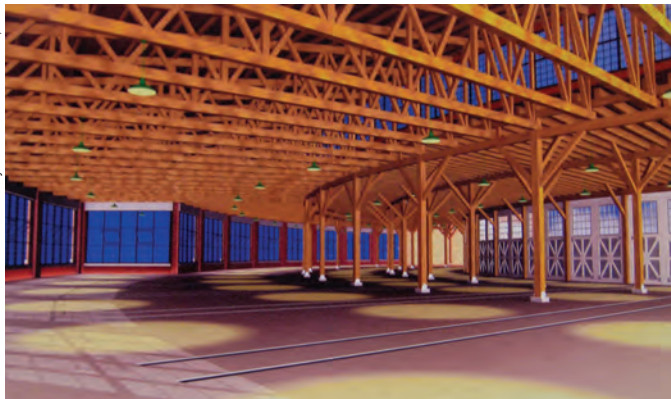
This architect's drawing of the interior of the roundhouse shows how massive 12x12 wooden timbers will be used in the construction of the building.
