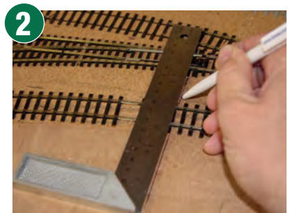
Mark a line along the cork in line with the tie bar.
