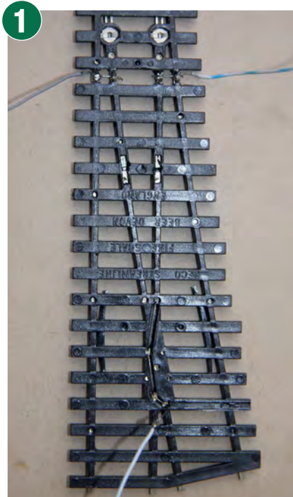
The underside of a Peco Electrofrog point with reliability modifications. The stock rail and switch rail are bonded on each side, with the wires leading to the accessory switch, and the two small factory fitted wires removed between the switch rails and the frog vee. The white wire from the frog will also lead to the accessory switch.
