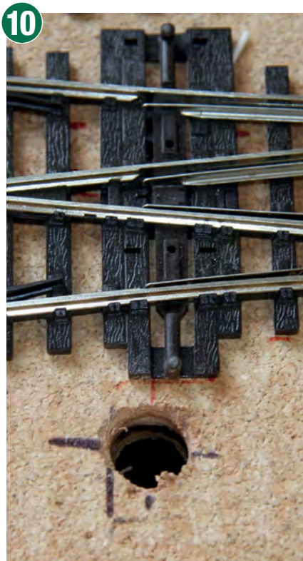
The 6mm hole has been drilled!
