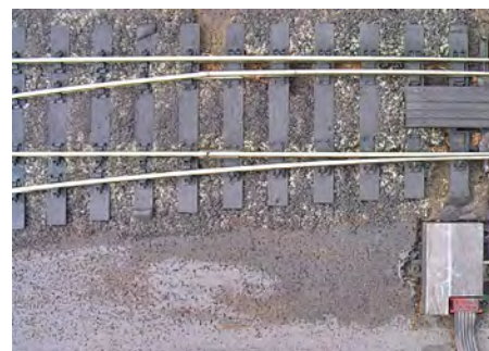
The small size of the unit makes it easy to disguise, unlike many larger point motors. The operating speed of the point can be varied over a wide range using a preset on the controller.
