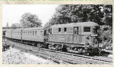
Number 17 was the first to be delivered and all 20 locomotives entered service circa 1922/23 - again, all official records have been lost. The solebar lifting lugs and fuse boxes swapped positions, the droplight cab front windows were sealed and two side windows were included by the single cab doors.
