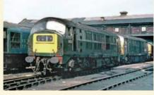
The 58 MAN-engined NBL Bo-Bos, built in 1958-60, became Class 21 under TOPS. The post-1966 Paxman-engined machines, illustrated by D6130 and D6137, parked in the sun at Eastfield on August 10 1969, were classified '29'. GORDON EDGAR/RAIL PHOTOPRINTS
