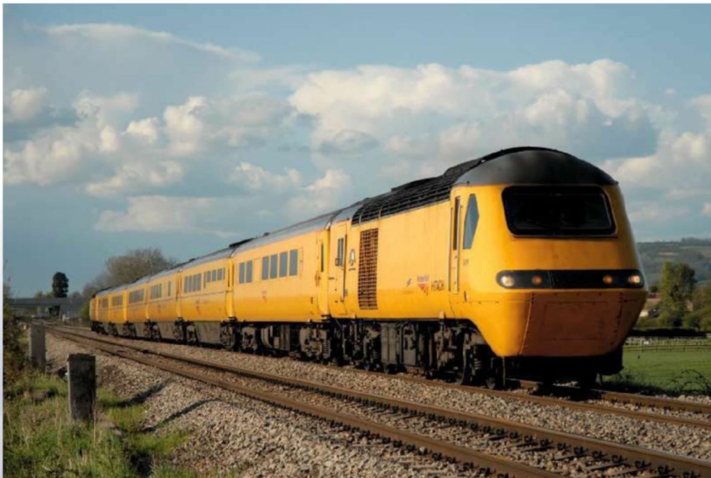
Network Rail has three HST power cars for its New Measurement Train. 43089 is the only one without nose-end buffing gear. It heads the NMT through Ashchurch on May 1 2008, having worked from Derby to Bristol Temple Meads via Paddington.
