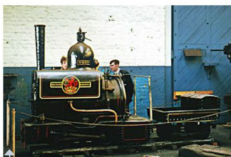
The smallest locomotive to wear mixed traffic black was Beyer Peacock 0-4-0VBT Wren. The post-1956 emblem almost covers the 18in gauge locomotive, which was built to work Horwich Works' internal railway network. D. FIELDING/COLOUR-RAIL
