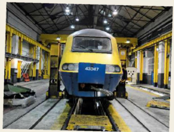
Above: EMT's 43047 inside Neville Hill's Back Fitting shop on December 8 2014. The power car shows off its front towing arrangement while it awaits engine replacement. PAUL BIGLAND/RAIL
