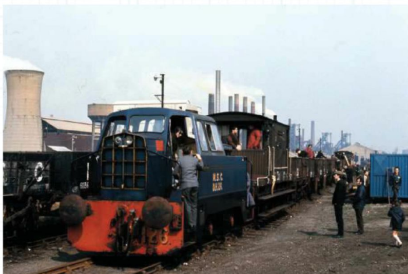
Above: MSC 26 works a brake van tour around the system in the 1970s. This was one of 14 Rolls-Royce Sentinel 4wDHs used on the railway. COLOUR RAIL
