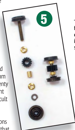
6 A wheel has to be removed from each axle and bearings, a washer and gear wheel slid on. Since the gear is too large for the axle, a tight fitting brass bush is carefully inserted into it.
