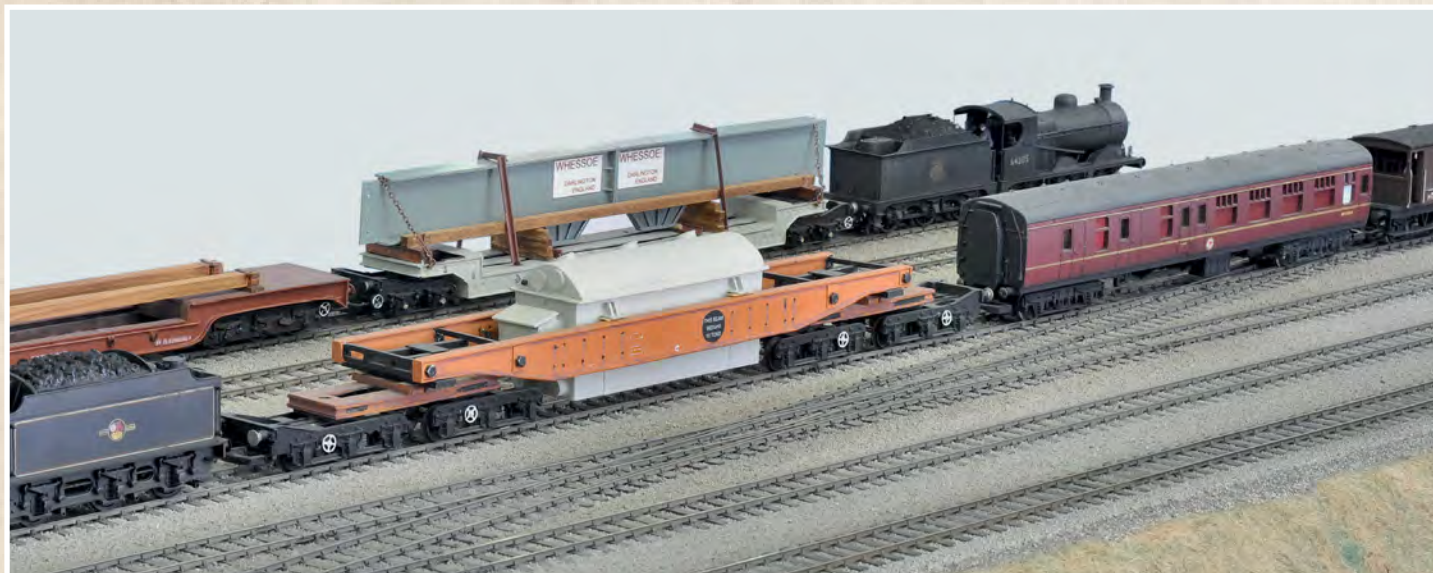
B901800/801 were a pair of 'Transformer MC' wagons built by Head Wrightson in 1953 to move heavy electrical equipment, one of which became the last specially constructed wagon in the BR revenue fleet, lasting until 1994. Harold's wagon is carrying a scratchbuilt industrial transformer. These wagons often ran under 'out of gauge' arrangements and if necessary could be rocked up to a foot either way to clear obstructions.
