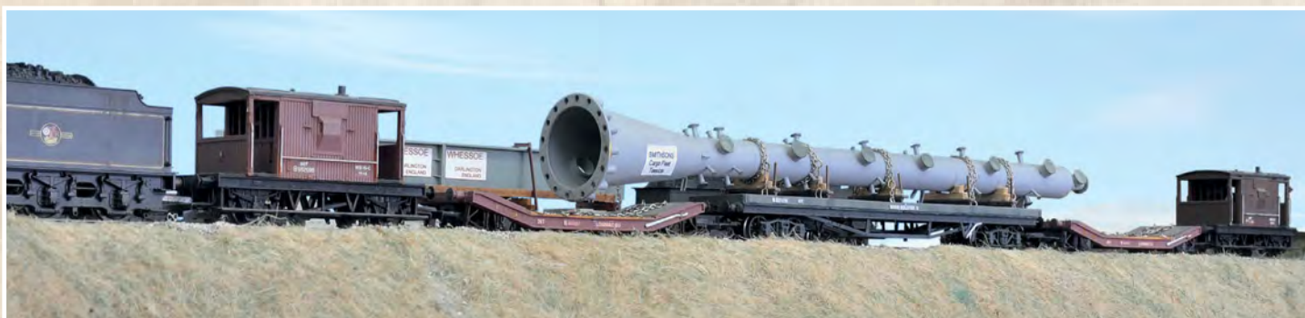
Being delivered from Smithson's in Cargo Fleet, near Middlesbrough, to a chemical works, this vertical boiler is mounted on a standard 'Bogie Bolster D' coupled between two 'Lowmac EU' barrier wagons. Exceptional loads had to be accommodated by railway companies when they had 'common carrier' status, before road haulage became more practical.
