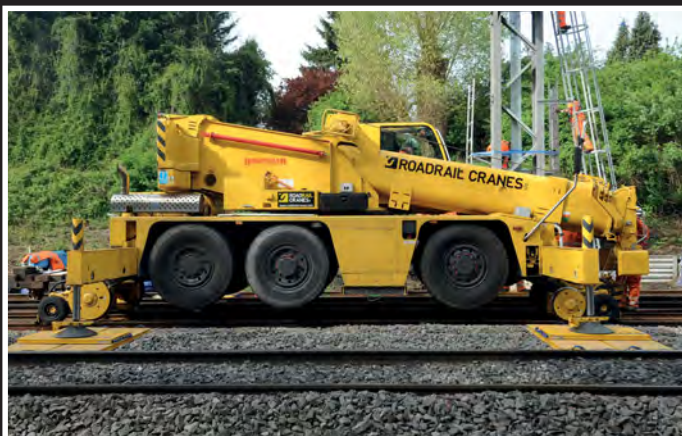
Proof that not all RRVs are small. Falling into the heavy-weight category of Road-Railers is this crane, operated by Roadrail cranes Ltd and seen at Hatch End on May 4, 2014.
