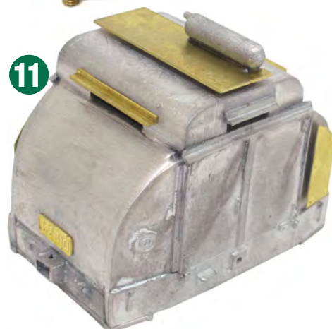
11 For the armoured locomotive, a solid top fits over the hole. A little filling and smoothing was required to finish the curved ends where they meet the sides.
