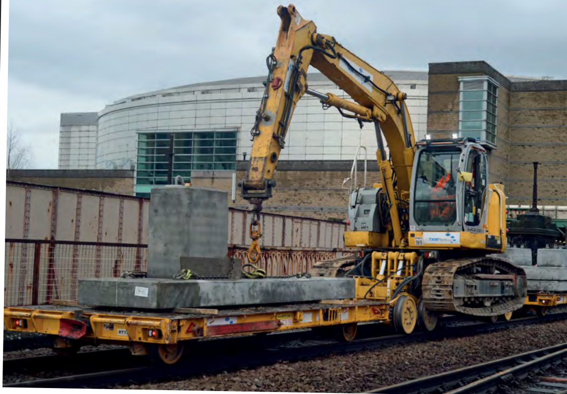
A New Holland-Kobelco E200SR is caught at Manchester Victoria 'top and tailed' by a pair of low wagons transporting overhead line electrification post foundation blocks. Such a compact setup replaces a main-line locomotive (using more fuel) and wagons.
