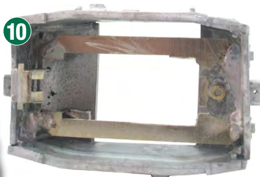
10 For speed I soldered the ends and sides of the whitmetal body together although epoxy or superglue will work just as well. The floor fits in here - check that the chassis still fits and is level. Getting it to sit low enough isn't easy - my model sits very slightly too high although this will allow it to handle less than perfect track.
