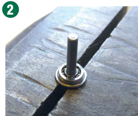
2 Both axles are driven via a layshaft on to which the worm gears are fitted as well as the pulley that takes drive from the motor. The shaft runs in a pair of ball-race bearings which are a very tight fit on the rod. Fit the bearing furthest from the pulley end. I supported this in a vice and tapped the shaft through gently with a small hammer.
