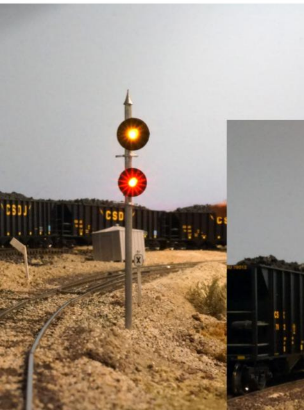
A signal cycles from green to red on the approach of a Santa Fe freight on Detlef Kurpanek's HO scale Great Northwestern layout. Detlef used Arduino microcontrollers to operate his signal system.
