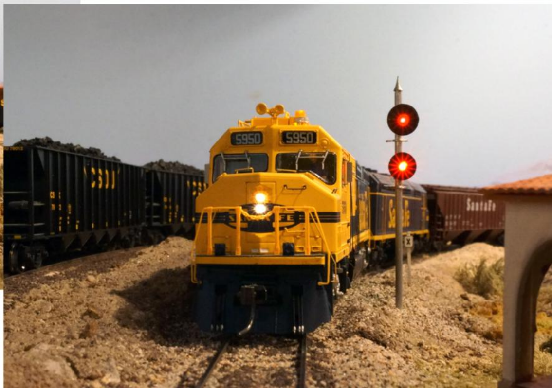
A signal cycles from green to red on the approach of a Santa Fe freight on Detlef Kurpanek's HO scale Great Northwestern layout. Detlef used Arduino microcontrollers to operate his signal system.
