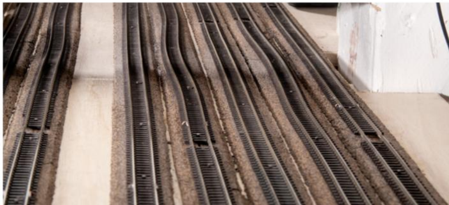
Kinks like these, seen on former Model Railroader managing editor Jim Kelly's N scale layout, can arise if you don't leave room for benchwork expansion and contraction in your rails. Jim Kelly photo
