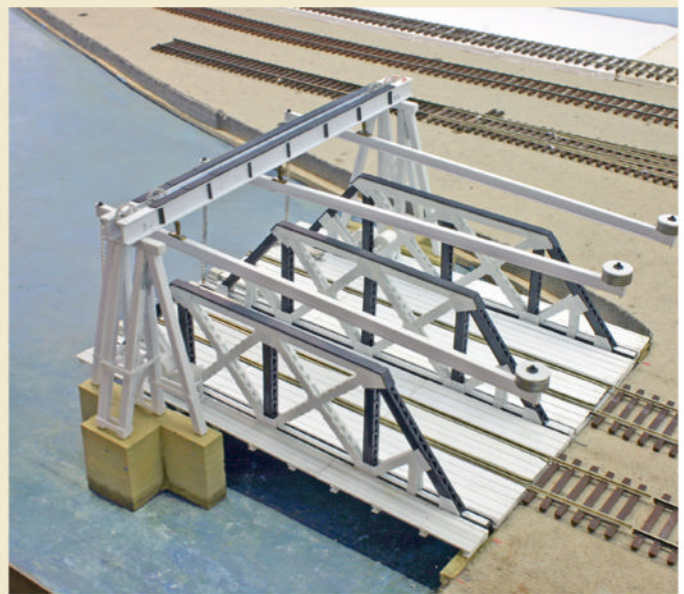
This transfer bridge is similar to a truss bridge and is built of styrene strip and shapes, plus some Central Valley truss bridge sections. Micro Engineering track was used on the deck and extends onto land, making it easier to solder feeder wires to power the rails.
