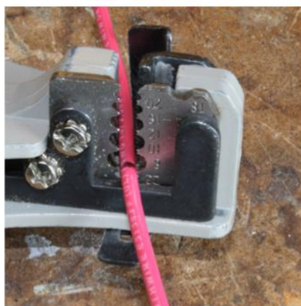
Fig. 4 In-line wire stripper. With the feeder locations marked, Pete set the wire in an in-line stripper. The blade makes the cut while the other side slides the insulation.
