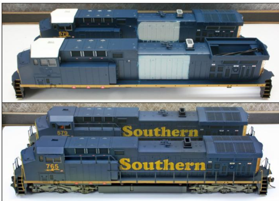
Fig. 6 Athearn GE AC4400CW. Bob had to remove the paint down to the raw plastic to get rid of the CSX herald on the Athearn models (top photo). This selective repainting allowed him to keep all of the factory applied warning stencils on the finished model (bottom photo).
