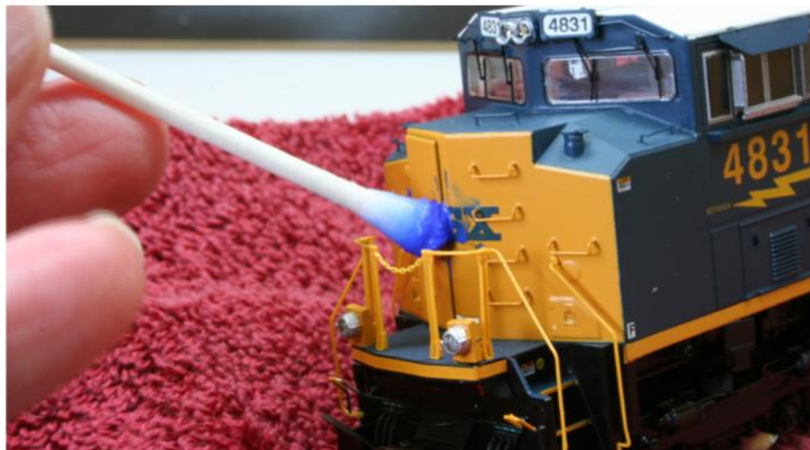
Fig. 1 Cotton swabs. Bob found that nothing was more effective at removing lettering than a cotton swab. Once the swab gets saturated with paint and starts smearing the surface, Bob would switch to a new one. He used several hundred swabs while redecorating the six locomotives in this article.
