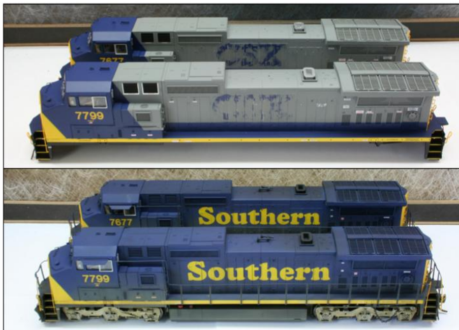
Fig. 5 Atlas GE Dash 8-40CW. Bob used isopropyl alcohol to remove most of the lettering from the model's long hood (top photo). He repainted the gray body (bottom photo) prior to applying his freelance decals.
