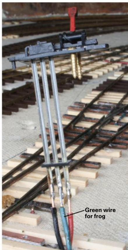
Fig. 9 Wiring ground throws. Pete used Caboose Industries ground throws with frog polarity contacts. The wiring followed the same protocol as the rest of his layout, with the addition of a green wire for the frog.
