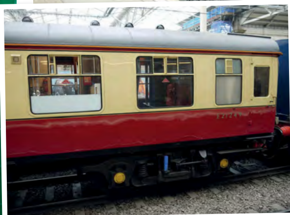
E21249 in more detail, showing the 'better than new' finish and additional equipment fitted to the extensively modernised Mk 1 coach. The compartment with the white panel is the new kitchen. BEN JONES
